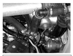
k. Install supplied 3/4" and 5/16" hoses onto inlet pipe as shown. Use supplied spring clamps and screw clamps as shown.
