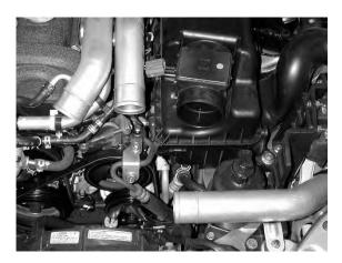
d. Remove the boost pipe elbow and the inlet tube. You will reuse the boost side elbow during the *AEM* intake install.
