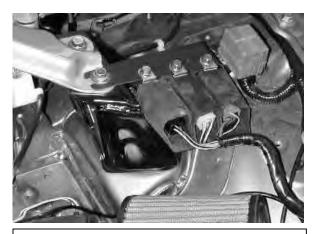
U) Attach relays to relay bracket using the stock M6 nuts and bolts from removal in step 2H as shown.
