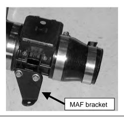
c. Assemble the supplied MAF bracket onto the MAF sensor as shown with the 2 M6 x 10 bolts removed in step 2L of disassembly. Install supplied 2.25" to 2.75" reducing coupler with clamps onto MAF sensor as shown. **Note:** Direction of MAF sensor!
