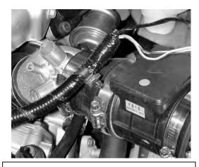
g. Remove the electrical tape as shown.
