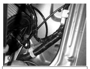
r. Cut and remove electrical tape on relay harness to give more length.
