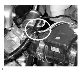
f. Cut electrical tape holding MAF wires to harness to give it extra length. Take care not to cut the wires.
