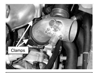
b. Install the supplied 1.75" to 2.25" reducing elbow coupler onto turbo inlet with pipe and clamps as shown.
