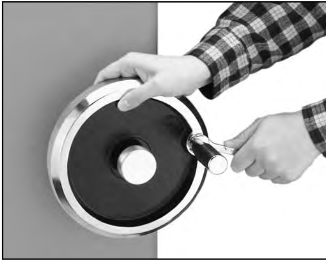
Figure 15. Tightening handle onto handwheel.
