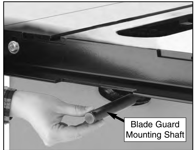
Figure 13. Attaching the \frac{5}{8} "-18 blade guard mounting shaft.
