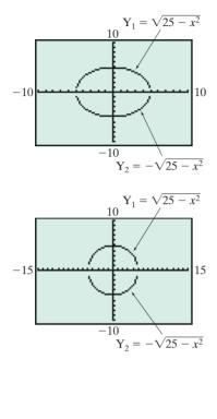
To graph an equation such as  $x^2 + y^2 = 25$  with a graphing calculator, we first solve the equation for *y*.
