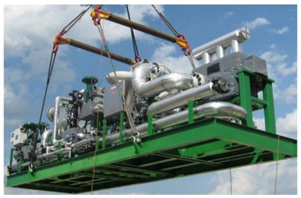
Echogen's first-of-kind EPS100 process skid being transported for testing.
