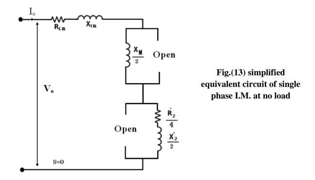
From the fig (13), the equivalent reactance at no load is given by
