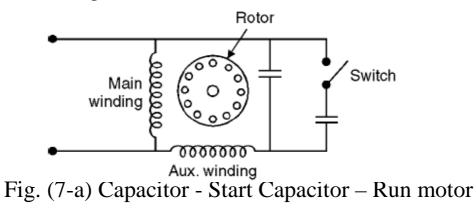
Theoretically, optimum starting and running performance can be achieved by having two capacitors. The starting capacitor is larger in value and is of the ac electrolytic type. The running capacitor permanently connected in series with the starting winding, is of smaller value and is of the paper oil type. Typical values of these capacitors for a 0.5 hp are  $C_s = 300\mu$ F,  $C_r = 40\mu$ F. The typical torque – speed characteristic is shown in fig. (7- b).
