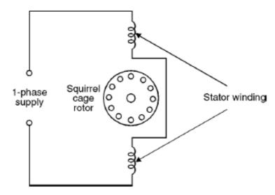
Fig. (1) Single – phase induction motor
