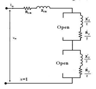
Fig.(12) simplified equivalent circuit of single phase I.M. with locked rotor
