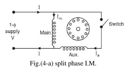
The auxiliary winding is made of thin wire so that it has a high R/X ratio as compared to the main winding which has thick super enamel copper wire. When the two stator windings are energized from a single – phase supply, the current  $I_m$  and  $I_a$  in the main winding and auxiliary winding lag behind the supply voltage V, and  $I_a$  leading the current  $I_m$  as shown in figure (4-b).
