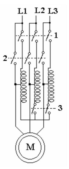
Fig.(3) shows I.M with auto transformer starter.
