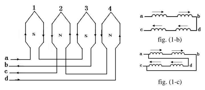
Fig. (1) Stator phase connections for 4 poles
