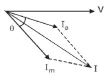
Fig.(4-b) Phasor diagram at starting
