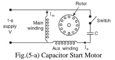
The value of capacitor is so chosen that  $I_a$  leads  $I_m$  by about 90° (Fig.5-b) so that the starting torque is maximum for certain values of  $I_a$  and  $I_m$ . Again, the starting winding is opened by the centrifugal switch when the motor attains about 75% of synchronous speed. The motor then operates as a single – phase induction motor and continues to accelerate till it reaches the normal speed.
