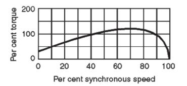
Fig.(8-b) torque – speed characteristic
