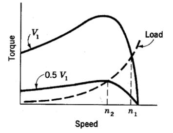
Fig. (3): Torque - speed curves for various terminal voltages
