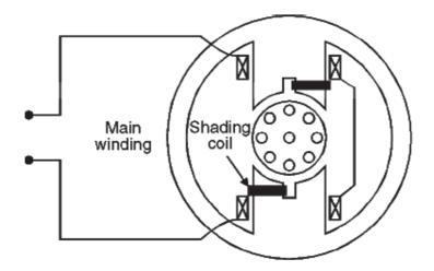
Fig (8-a) Shaded Pole Induction Motor
