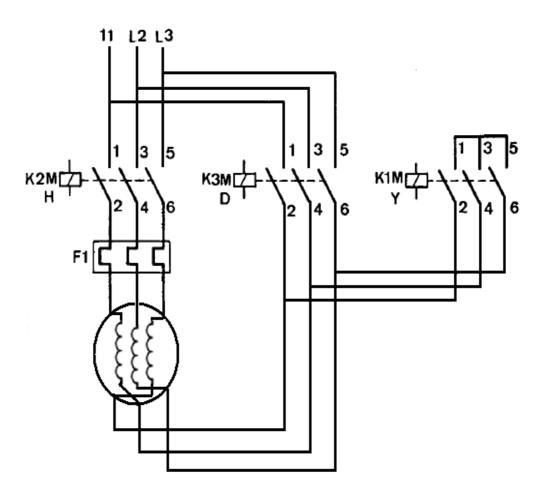
Fig.(2) Induction Motor with Star Delta Starter
