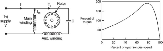
Fig.(6-a) Permanent – Split Capacitor Motor
