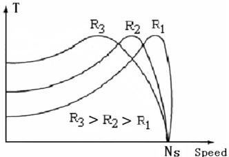
Fig.(4) Torque – speed curve for rotor resistance variation
