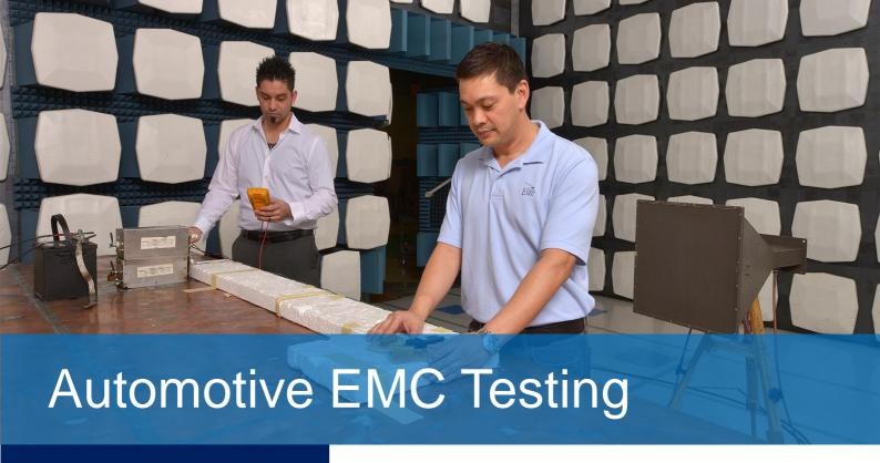
Automotive EMC testing measures the radio frequency (RF) emissions emanating from vehicle electrical systems and evaluates their susceptibility to RF signals generated by other devices on the vehicle as well as from offvehicle sources.
