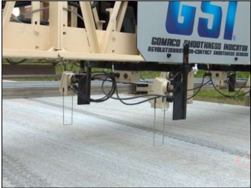
Figure 78 – Noncontact smoothness profile equipment (GOMACO)
