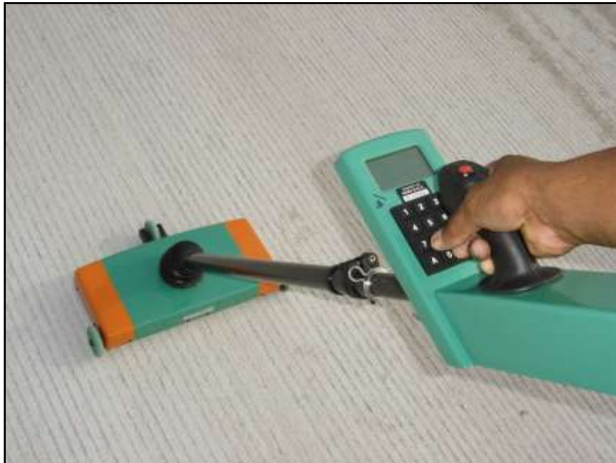
Figure 81 – Nondestructive pavement thickness equipment (MIT-SCAN-T2)
