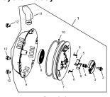
Description APGG1000-G-01-JD RECOIL STARTER ASSY APG3090-G-02-JD SETTING SCREW APG3090-G-03-JD SPRING RETAINER APG3090-G-04-JD PLATEN SPRING APG3090-G-05-JD STARTER RATCHET APG3090-G-06-JD RETURN SPRING APG3090-G-07-JD RECOIL STARTER REEL APG3090-G-08-JD RECOIL STARTER SPRING APGG10000-G-09-JD RECOIL STARTER CASE COMP RECOIL STARTER ROPE APG3090-G-10-JD APG3090-G-11-JD STARTER KNOB APG3090-G-12-JD FLANGE BOLT (M6X8)
