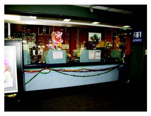
**Figure 11** 3.013 – The RTA registry counter does not have an accessible section for a person with disabilities. The seated section is for persons undergoing testing. An accessible new toilet may be required in the foyer for the public (SPA to confirm).
