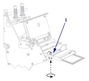
19. Push down the printhead assembly (1), and then rotate the printhead-open lever (2) until it locks into place.
