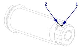
**3.** Align the segments of the ribbon supply spindle.
