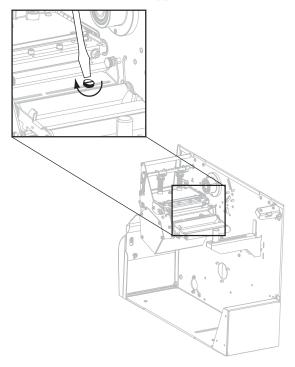
6. Adjust the lower media sensor to match the new position of the upper media sensor. See Lower Media Sensor on page 118.
