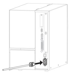
2. Plug the male end of the A/C power cord into an appropriate power outlet.
