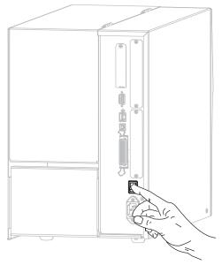
The printer boots up and performs a self-test.
