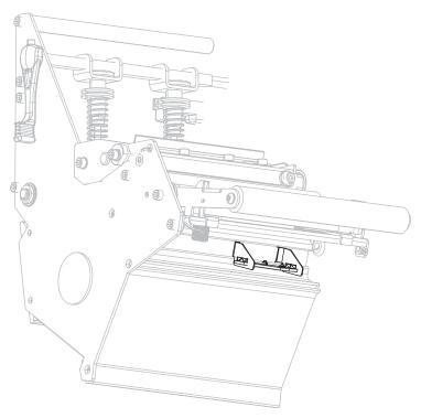
**2.** Slide the lower sensor until it is under the upper media sensor. Use the light that shines from the lower sensor to help align it with the upper sensor. Gently pull the wires as needed (wires should have a little slack).
