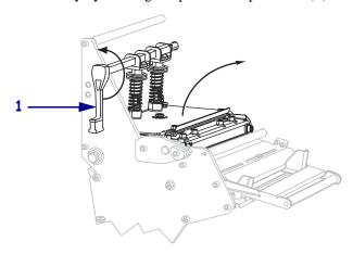
2. Loosen the thumb screw (not visible from this angle) that is located on the bottom of the outer media guide (1).
