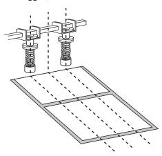
**5.** Tighten the locking nuts.
