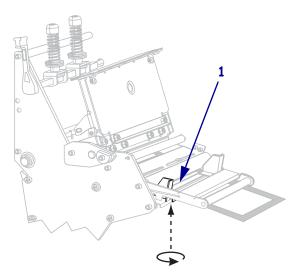
**15.** Push down the printhead assembly (1), and then rotate the printhead-open lever (2) until it locks into place.
