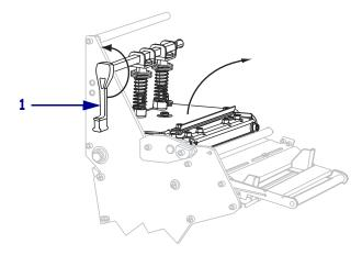
**8.** Thread the ribbon over the media dancer assembly (1) and under the ribbon guide roller (2).
