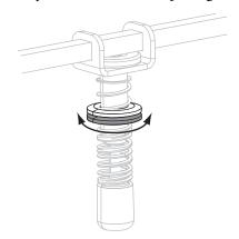
**5.** To lock the toggle pressure, tighten the locking nut against the adjusting nut.
