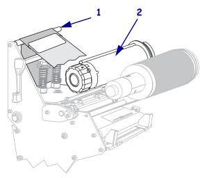
**11.** Wind the ribbon leader and attached ribbon counterclockwise around the ribbon take-up spindle.
