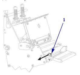
4. Insert media into the printer. Follow the instructions for roll or fanfold media, as appropriate.
