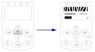
At the Idle Display (Figure 3), press **SETUP** to enter Setup Mode. The printer displays the first parameter.
