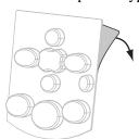
2. Carefully align the cover over the keypad. Press to make the cover adhere to the printer.
