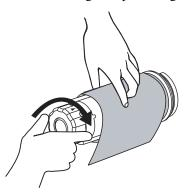
3. Slide the used ribbon off of the ribbon take-up spindle and discard.
