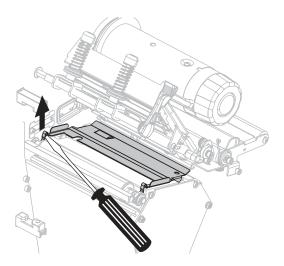
**4.** Insert the small-blade screwdriver or similar tool into the loop on the right side of the snap plate. Gently lift the right side of the snap plate.
