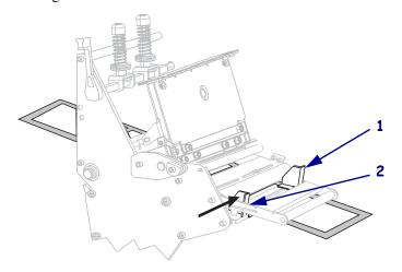
**10.** Tighten the thumb screw (not visible from this angle) that is located on the bottom of the outer media guide (**1**).
