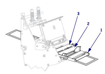
**6.** Push the media forward until it passes under the printhead assembly (1), under the snap plate (2), and then over the platen roller (3).
