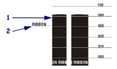
Media Sensor Profile (Figure 20) The media sensor readings are shown as bars and flat areas on the sensor profile (Figure 20). The bars (1) indicate gaps between labels (the web), and the low areas (2) indicate where labels are located. If you compare the sensor profile printout to a blank length of your media, the bars should be the same distance apart as the gaps on the media. If the distances are not the same, the printer may be having difficulty determining where the gaps are located.
