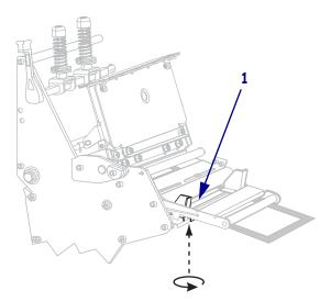
**10.** Push down the printhead assembly (1), and then rotate the printhead-open lever (2) until it locks into place.
