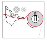
8. Align the media with the inner media guide (1). Slide in the outer media guide (2) until it just touches the edge of the media.
