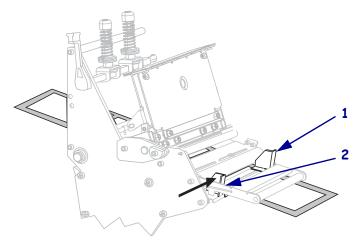
**18.** Tighten the thumb screw (not visible from this angle) that is located on the bottom of the outer media guide (1).
