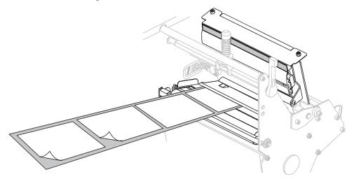
**10.** Remove the hook from the rewind spindle.
