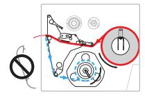
**8.** Remove the rewind plate (if installed) from the front of the printer. Store it on the two mounting screws on the inside of the printer base.
