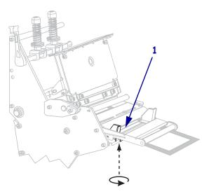
**11.** Push down the printhead assembly (1), and then rotate the printhead-open lever (2) until it locks into place.
