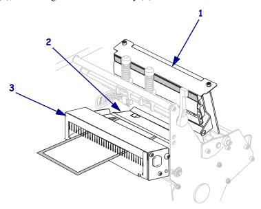
9. Align the media with the inner media guide (1). Slide in the outer media guide (2) until it just touches the edge of the media.
