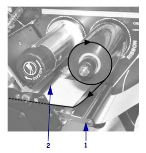
**9.** Push the ribbon leader forward until it passes under the printhead assembly (1), over the snap plate (2), and then over the platen roller (3).
