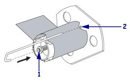
**b.** Rotate the spindle counterclockwise several turns to wind the media liner over the hook and remove any slack.
