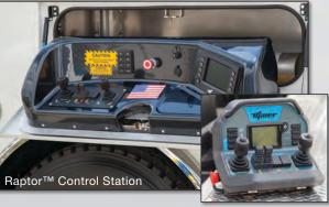
The operator can easily maneuver through operations at the unit control station or on the wireless remote.
