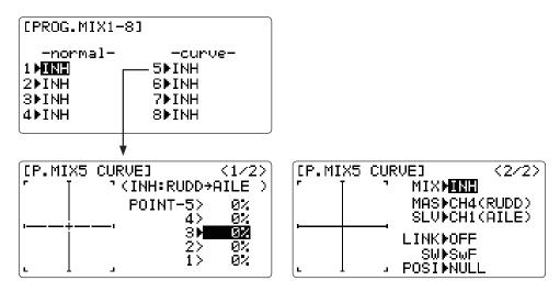
Your 10CG's **ACRO/GLID** programs contain four separate curve programmable mixes. **HELI** contains two. There are a variety of reasons you might want curve mixes. For example when a linear mix doesn't fit your needs along the whole range. One pre-programmed curve mix is the **THROTTLE-NEEDLE** function. This curve is adjustable at 5 points, allowing you to adjust the motor's tuning at 5 points along its RPM range.
