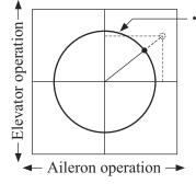
•Swash travel by simultaneous operation of the ailerons and elevators is limited within the circle(**SWASH RING** rate).
