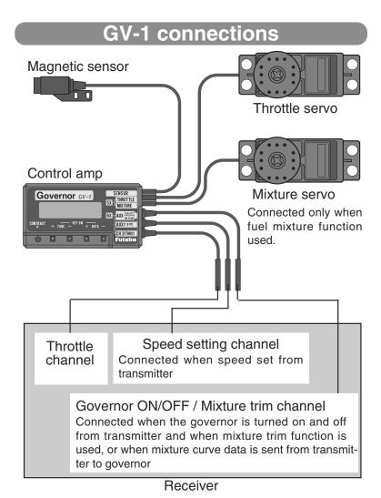
What is a governor? A governor is made up of a set of sensors which read the RPM of the helicopter's head, and a control unit that automatically adjusts the throttle setting to maintain a constant head speed regardless of changes in pitch of blades, weather conditions, etc. Governors are extremely popular in competition helicopters due to the consistency provided.
