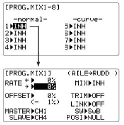
Your 10CG contains four separate linear programmable mixes. (Note that mixer #5-8's mixing **RATEs** are set with a 5-point curve. **HELI** has mixer #5-6's mixing. see CURVE MIXES, p. 71.)
