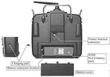
NOTE: If you need to remove or replace the transmitter battery, do not pull on its wires to remove it. Instead, gently pull on the connector's plastic housing where it plugs into the transmitter.
