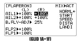
The **FLAPERON** mixing function uses one servo on each of the two ailerons, and uses them for both aileron and flap function. For flap effect, the ailerons raise/lower simultaneously. Of course, aileron function (moving in opposite directions) is also performed.
