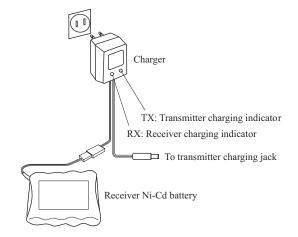
The initial charge, and any charge after a complete discharge, should be at least 18 hours to ensure full charge. The batteries should be left on charge for about 15 hours when recharging the standard NR-4J, NR4F1500 and NT8S700B Ni-Cd batteries.
