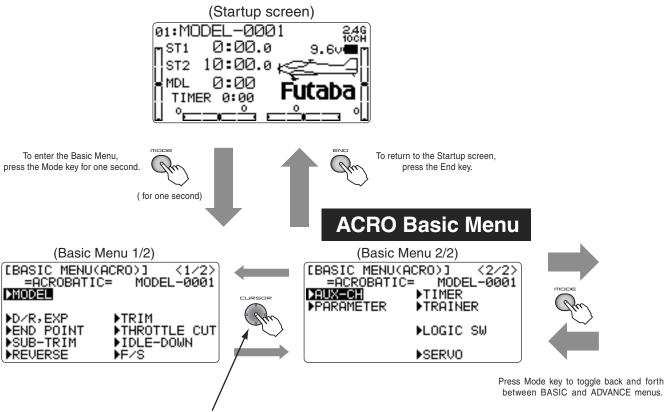
Press Cursor lever to page up and down through the 2 pages of screens in each menu. Note that all functions which have more than one page have a <1/2> indicator in the upper right hand corner to indicate page 1 of 2 or page 2 of 2.
