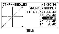
**THROTTLE STICK** inputs for perfect engine tuning at all throttle settings. This function is particularly popular with contest pilots who fly in a large variety of locations, needing regular engine tuning adjustments, and requiring perfect engine response at all times and in all maneuvers. Also popular to minimize flooding at idle of inverted engine installations or installations with a high tank position. Not needed for fuel injection engines, which do this automatically.
