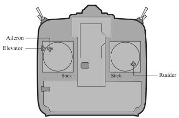
Mode 2 transmitter with rear cover removed.
