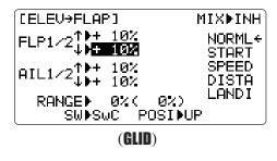
**ELEV-FLAP** mixing is the first pre-programmed mix we'll cover. This mix makes the flaps drop or rise whenever the *ELEVATOR STICK* is moved. It is most commonly used to make tighter pylon turns or squarer corners in maneuvers. In most cases, the flaps droop (are lowered) when up elevator is commanded.
