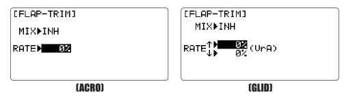
**FLAP-TRIM** assigns the primary flaperon control [defaults to VR(A)] to allow trimming in flight of the flap action of flaperons. (Note: even if **FLAP-TRIM** is made active with **All-DIFF**, it will not have any effect. The ONLY function that allows control of the ailerons as flaps in the **All-DIFF** configuration is **AIRBRAKE**.) Most modelers use **AIRBRAKE**, or programmable mixes, to move the flaps to a specified position via movement of a switch.
