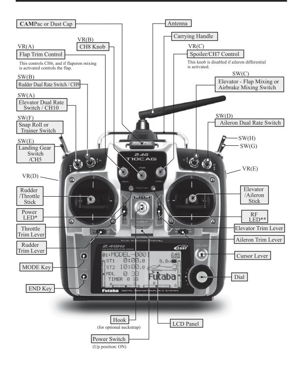
This figure shows the default switch assignments for a 10CAG Mode 2 system as supplied by the factory. You can change many of the switch positions or functions by selecting a new position within the setting menu for the function you wish to move. (Example: move aileron dual rates to switch C to create triple rates. See p. 42 for details.)
