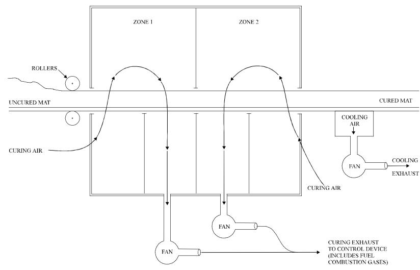
Figure 11.13-3. Side view of curing oven (indirect heating) and cooling section.
