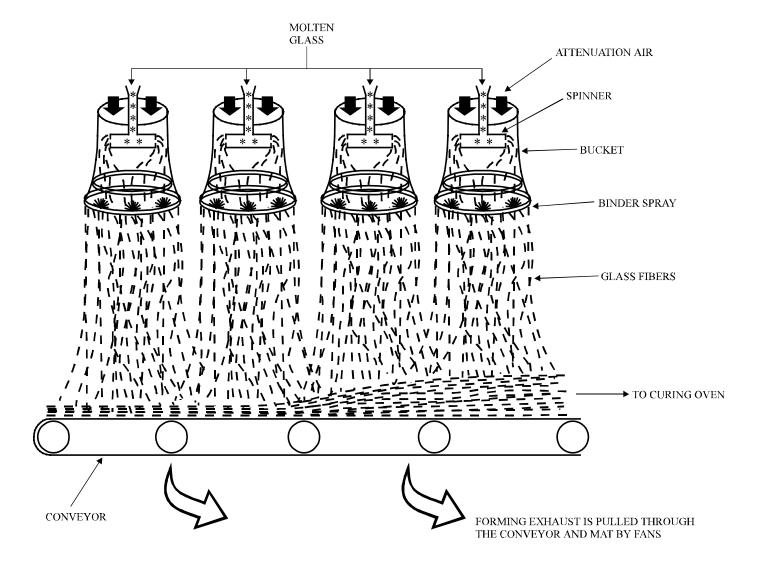
Figure 11.13-2. A typical spin process.
