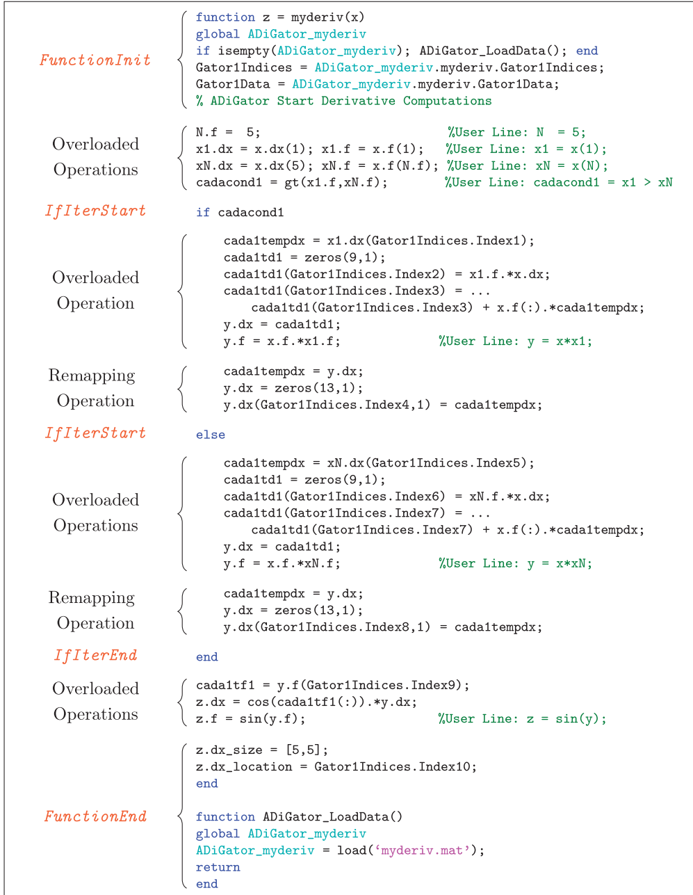
Fig. 12. Transformed derivative program for Example 1 showing from where each line is printed.
