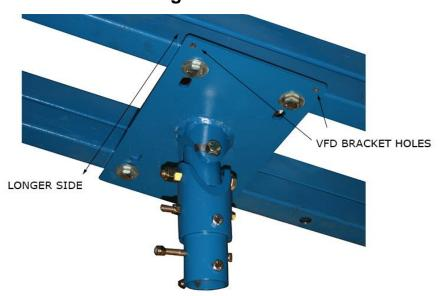
v) If a down rod was ordered, remove the 4¾" connector and replace with the longer down rod. Refer to Image 2.
