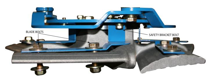
D) Install blade flaps using  $\frac{1}{4}$ " bolts and end caps using #10 x  $\frac{1}{2}$ " screws provided. Ensure  $\frac{1}{4}$ " bolts are tight on flaps. The pan head of the bolts go into the countersinks in the bottom of the blades. Refer to Image 14 for more information.
