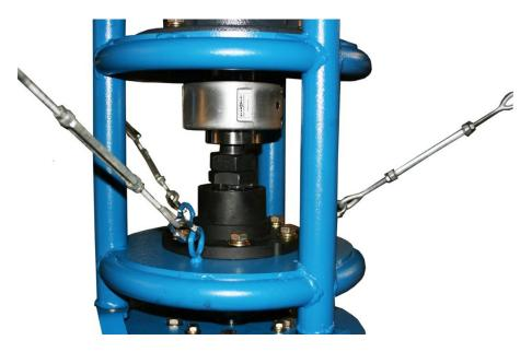
A) Attach the looped end of the guy wire to the turnbuckle located on the fan assembly. It should appear like the Image 10.
