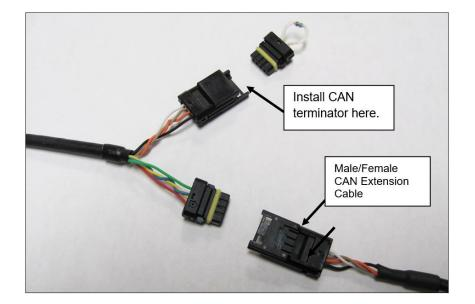
Holley EFI main harnesses use two types of CAN connectors. Earlier harnesses use a 2 pin metripak connector. The kit includes an adapter to go from this to the 4' extension harness (note the white power and black ground wires are NOT needed for the Pro Dash, but need to be connected if other CAN devices require it for their power supply). Later harnesses plug directly into the 4' extension harness.
