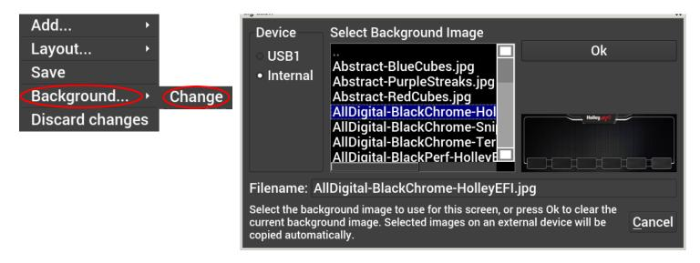
To remove the background from the current layout, press Ok without selecting a filename.
