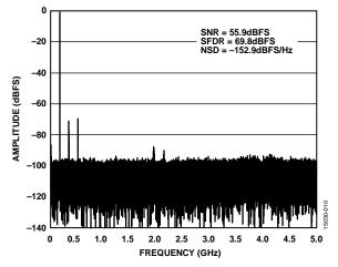
Figure 38. Single-Tone FFT with  $f_{IN} = 170$  MHz, 10 GSPS
