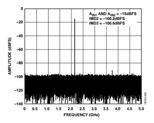
Figure 68. Two-Tone FFT,  $f_{\rm IN1} = 2137.5$  MHz,  $f_{\rm IN2} = 2142.5$  MHz,  $A_{\rm IN1}$  and  $A_{\rm IN2} = -15$  dBFS, 10 GSPS
