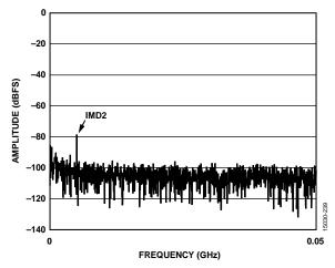
Figure 24. Two-Tone FFT, IMD2 Zoom In,  $f_{\rm IN1}=1841.5~{\rm MHz}, f_{\rm IN2}=1846.5~{\rm MHz},$   $A_{\rm IN1}~and~A_{\rm IN2}=-7~{\rm dBFS}$  (see Figure 23), 6 GSPS
