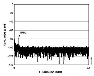
Figure 28. Two-Tone FFT, IMD2 Zoom In,  $f_{\rm IN1}=2137.5$  MHz,  $f_{\rm IN2}=2142.5$  MHz,  $A_{\rm IN1}$  and  $A_{\rm IN2}=-7$  dBFS, 6 GSPS
