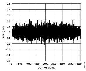
Figure 32. DNL at  $f_{IN} = 170 \text{ MHz}$ , 6 GSPS
