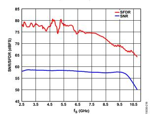
Figure 48. SNR/SFDR vs. Sampling Frequency,  $f_{IN} = 170 \text{ MHz}$
