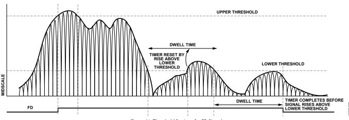
Figure 91. Threshold Settings for FD Signal
