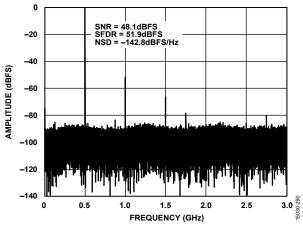
Figure 12. Single-Tone FFT with  $f_{IN} = 5.5$  GHz, 6 GSPS
