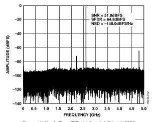
Figure 40. Single-Tone FFT with  $f_{\text{IN}}$  = 2.6 GHz, 10 GSPS
