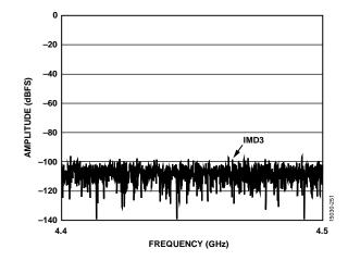
Figure 64. Two-Tone FFT, IMD3 Zoom In,  $f_{\rm IN1} = 1841.5$  MHz,  $f_{\rm IN2} = 1846.5$  MHz,  $A_{\rm IN1}$  and  $A_{\rm IN2} = -15$  dBFS (see Figure 62), 10 GSPS
