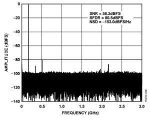
Figure 6. Single-Tone FFT with  $f_{IN} = 170$  MHz, 6 GSPS
