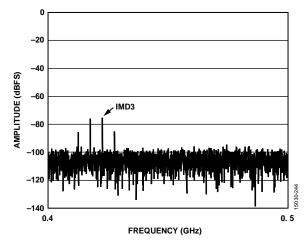
Figure 29. Two-Tone FFT, IMD3 Zoom In,  $f_{\rm IN1}$  = 2137.5 MHz,  $f_{\rm IN2}$  = 2142.5 MHz,  $A_{\rm IN1}$  and  $A_{\rm IN2}$  = -7 dBFS, 6 GSPS
