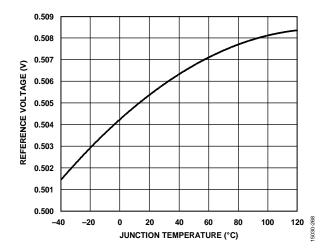
Figure 75. Reference Voltage vs. Junction Temperature, 10 GSPS
