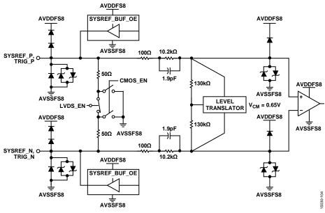
Figure 87. SYSREF\_x and TRIG\_x Inputs
