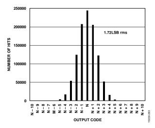
Figure 71. Input-Referred Noise Histogram, 10 GSPS
