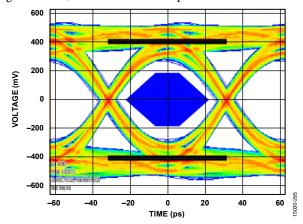
Figure 119. Digital Outputs Data Eye, External 100  $\Omega$  Terminations at 16 Gbps
