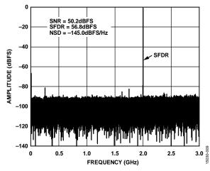
Figure 9. Single-Tone FFT with  $f_{IN} = 4$  GHz, 6 GSPS
