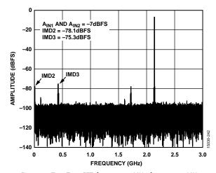
Figure 27. Two-Tone FFT,  $f_{\rm IN1}=2137.5$  MHz,  $f_{\rm IN2}=2142.5$  MHz,  $A_{\rm IN1}$  and  $A_{\rm IN2}=-7$  dBFS, 6 GSPS
