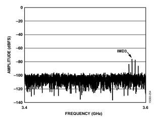
Figure 67. Two-Tone FFT, IMD3 Zoom In,  $f_{\text{IN1}} = 2137.5 \text{ MHz}$ ,  $f_{\text{IN2}} = 2142.5 \text{ MHz}$ ,  $A_{\text{IN1}}$  and  $A_{\text{IN2}} = -7 \text{ dBFS}$  (see Figure 65), 10 GSPS
