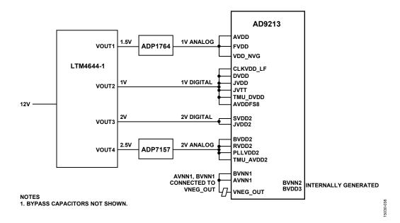
Figure 126. Alternate Simplified Power Supply Configuration
