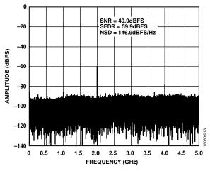
Figure 41. Single-Tone FFT with  $f_{IN} = 4$  GHz, 10 GSPS
