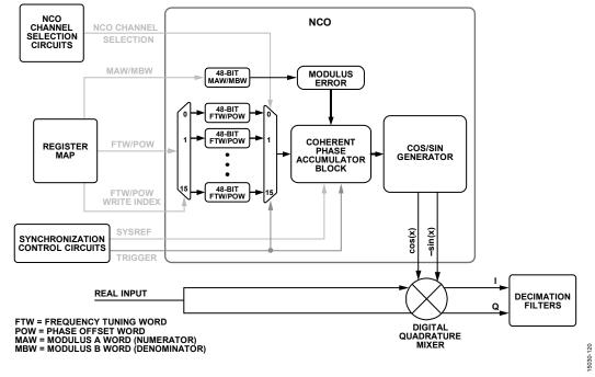
Figure 95. NCO and Mixer Block Diagram
