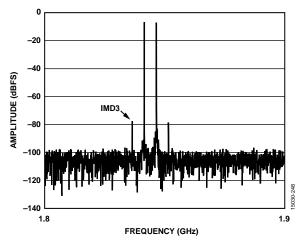
Figure 60. Two-Tone FFT, IMD3 Zoom In,  $f_{\rm IN1}=1841.5$  MHz,  $f_{\rm IN2}=1846.5$  MHz,  $A_{\rm IN1}$  and  $A_{\rm IN2}=-7$  dBFS (see Figure 59), 10 GSPS
