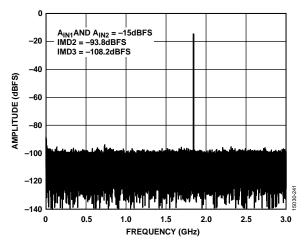
Figure 26. Two-Tone FFT,  $f_{\rm IN1} = 1841.5$  MHz,  $f_{\rm IN2} = 1846.5$  MHz,  $A_{\rm IN1}$  and  $A_{\rm IN2} = -15$  dBFS, 6 GSPS
