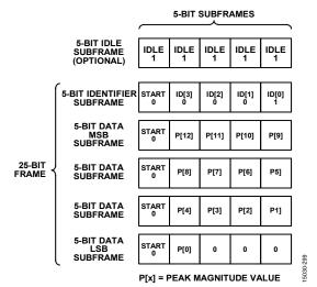
Figure 112. SPORT over JESD204B Signal Monitor Frame Data
