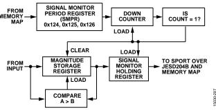
Figure 110. Signal Monitor Block
