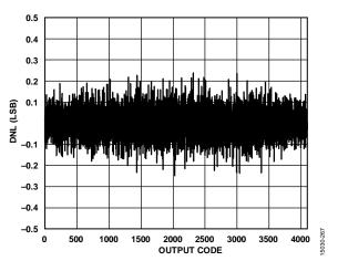
Figure 69. DNL at  $f_{IN} = 170 \text{ MHz}$ , 10 GSPS
