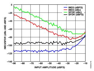
Figure 72. IMD3/SFDR vs. Input Amplitude,  $f_{\rm IN1}$  = 2137.5 MHz,  $f_{\rm IN2}$  = 2142.5 MHz, 10 GSPS
