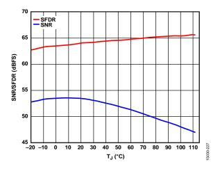
Figure 57. SNR/SFDR vs.  $T_J$ ,  $f_{IN} = 2600$  MHz, 10 GSPS
