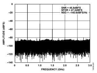
Figure 13. Single-Tone FFT with  $f_{IN} = 6.5$  GHz, 6 GSPS
