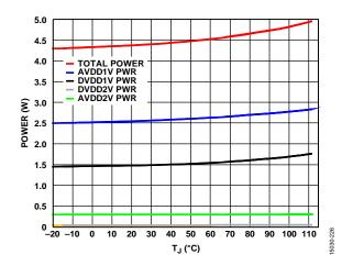
Figure 58. Power vs.  $T_{J}$ ,  $f_{IN} = 2600 \text{ MHz}$ , 10 GSPS
