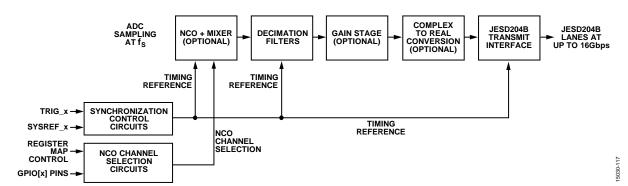
Figure 92. DDC Detailed Block Diagram
