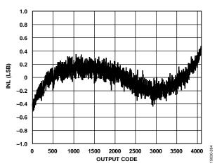
Figure 31. INL at  $f_{IN} = 170$  MHz, 6 GSPS
