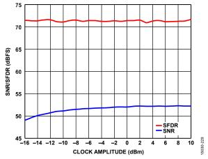
Figure 21. SNR/SFDR vs. Clock Amplitude at  $f_{IN} = 2600$  MHz, 6 GSPS
