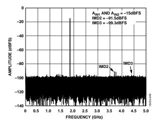
Figure 62. Two-Tone FFT,  $f_{\rm IN1}$  = 1841.5 MHz,  $f_{\rm IN2}$  = 1846.5 MHz,  $A_{\rm IN1}$  and  $A_{\rm IN2}$  = -15 dBFS, 10 GSPS
