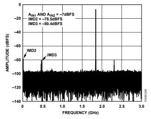
Figure 23. Two-Tone FFT,  $f_{\rm IN1}=1841.5~{\rm MHz}, f_{\rm IN2}=1846.5~{\rm MHz},$   $A_{\rm IN1}~and~A_{\rm IN2}=-7~dBFS, 6~GSPS$
