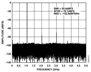
Figure 39. Single-Tone FFT with  $f_{IN} = 1$  GHz, 10 GSPS
