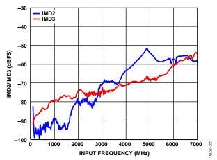
Figure 34. IMD2/IMD3 vs. Input Frequency ( $A_{\rm IN} = -7 {\rm dBFS}$ ), 10 MHz Spacing, 6 GSPS
