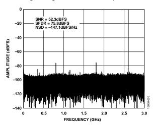
Figure 8. Single-Tone FFT with  $f_{IN} = 2.6$  GHz, 6 GSPS
