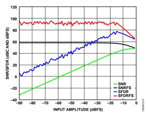
Figure 52. SNR/SFDR vs. Input Amplitude (A<sub>IN</sub>),  $f_{IN} = 2600$  MHz, 10 GSPS
