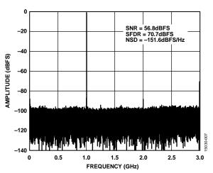
Figure 7. Single-Tone FFT with  $f_{IN} = 1$  GHz, 6 GSPS
