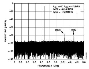
Figure 65. Two-Tone FFT,  $f_{\text{IN1}} = 2137.5$  MHz,  $f_{\text{IN2}} = 2142.5$  MHz,  $A_{\text{IN1}}$  and  $A_{\text{IN2}} = -7$  dBFS, 10 GSPS
