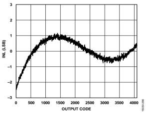
Figure 70. INL at  $f_{IN} = 170 \text{ MHz}$ , 10 GSPS
