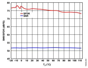
Figure 37. SNR/SFDR vs.  $T_J$ ,  $f_{IN} = 2600$  MHz, 6 GSPS
