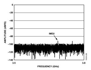
Figure 63. Two-Tone FFT, IMD2 Zoom In,  $f_{\rm IN1}=1841.5$  MHz,  $f_{\rm IN2}=1846.5$  MHz,  $A_{\rm IN1}$  and  $A_{\rm IN2}=-15$  dBFS (see Figure 62), 10 GSPS
