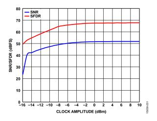
Figure 56. SNR/SFDR vs. Clock Amplitude,  $f_{IN} = 2600 \text{ MHz}$ , 10 GSPS
