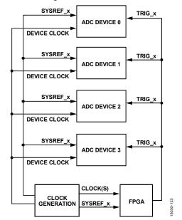
Figure 98. System Using TRIG\_x and SYSREF\_x for Synchronization
