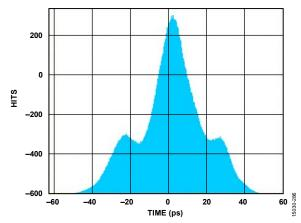
Figure 120. Digital Outputs Histogram, External 100  $\Omega$  Terminations at 16 Gbps
