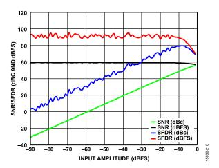
Figure 17. SNR/SFDR vs. Input Amplitude,  $f_{IN} = 1000$  MHz, 6 GSPS
