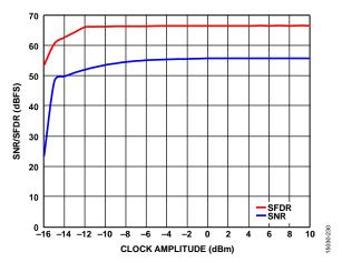
Figure 55. SNR/SFDR vs. Clock Amplitude,  $f_{IN} = 1000 \text{ MHz}$ , 10 GSPS
