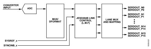
Figure 114. Transmit Link Simplified Block Diagram Showing Full Bandwidth Mode (Register 0x606 = 0x00)
