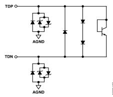
Figure 80. TDx Temperature Diodes
