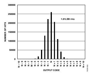
Figure 33. Input Referred Noise Histogram, 6 GSPS
