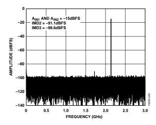
Figure 30. Two-Tone FFT,  $f_{\rm IN1}=2137.5$  MHz,  $f_{\rm IN2}=2142.5$  MHz,  $A_{\rm IN1}$  and  $A_{\rm IN2}=-15$  dBFS, 6 GSPS
