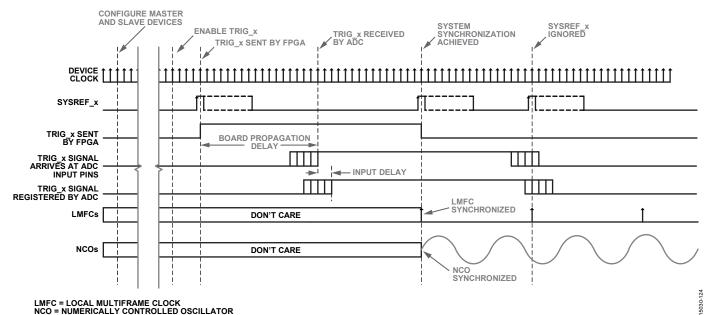
Figure 99. NCO Multichip Synchronization at Startup (Using TRIG\_x and SYSREF\_x)
