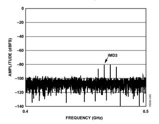
Figure 25. Two-Tone FFT, IMD3 Zoom In,  $f_{\text{IN1}} = 1841.5 \text{ MHz}$ ,  $f_{\text{IN2}} = 1846.5 \text{ MHz}$ ,  $A_{\text{IN1}}$  and  $A_{\text{IN2}} = -7 \text{ dBFS}$  (see Figure 23), 6 GSPS
