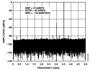
Figure 43. Single-Tone FFT with  $f_{IN} = 6.5$  GHz, 10 GSPS
