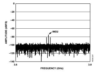
Figure 61. Two-Tone FFT, IMD2 Zoom In,  $f_{\text{IN1}} = 1841.5 \text{ MHz}$ ,  $f_{\text{IN2}} = 1846.5 \text{ MHz}$ ,  $A_{\text{IN1}}$  and  $A_{\text{IN2}} = -7 \text{ dBFS}$  (see Figure 59), 10 GSPS
