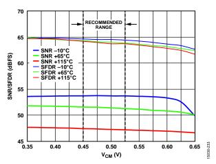
Figure 54. SNR/SFDR vs.  $V_{CM}$ ,  $f_{IN} = 2600$  MHz, 10 GSPS, Temperatures Shown =  $T_J$
