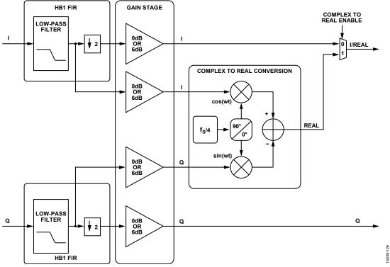
Figure 109. Complex to Real Conversion Block
