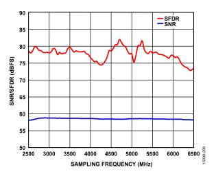
Figure 14. SNR/SFDR vs. Sampling Frequency,  $f_{IN} = 170 \text{ MHz}$ , 6 GSPS
