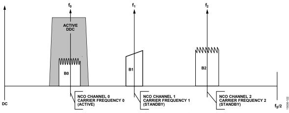
Figure 97. NCO Coherent Mode with Three NCO Channels (B0 Selected)
