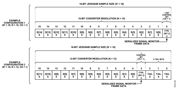
Figure 111. Signal Monitor Control Bit Location
