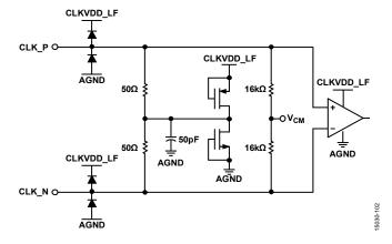
Figure 78. Clock Inputs
