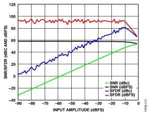
Figure 51. SNR/SFDR vs. Input Amplitude,  $f_{\rm IN}$  = 1000 MHz, 10 GSPS
