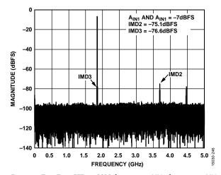
Figure 59. Two-Tone FFT, 10 GSPS,  $f_{\rm IN1} = 1841.5$  MHz,  $f_{\rm IN2} = 1846.5$  MHz,  $A_{\rm IN1}$  and  $A_{\rm IN2} = -7$  dBFS
