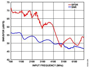
Figure 53. SNR/SFDR vs. Input Frequency ( $f_{IN}$ ), 10 GSPS,  $A_{IN} = -1$  dBFS
