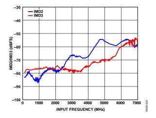
Figure 74. IMD2/IMD3 vs. Input Frequency ( $A_{\rm IN} = -7$  dBFS), 10 MHz Spacing, 10 GSPS
