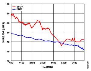
Figure 19. SNR/SFDR vs.  $f_{IN}$ ,  $A_{IN} = -1$  dBFS, 6 GSPS
