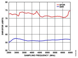
Figure 15. SNR/SFDR vs. Sampling Frequency,  $f_{IN} = 1000$  MHz, 6 GSPS
