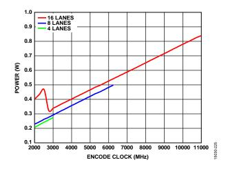
Figure 47. Power vs. Encode Clock (fs) for a Various Number of JESD204B Lanes, f<sub>IN</sub> = 170 MHz, 10 GSPS
