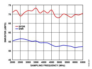
Figure 16. SNR/SFDR vs. Sampling Frequency,  $f_{IN} = 2.6$  GHz, 6 GSPS
