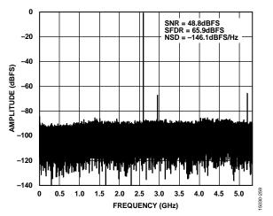
Figure 45. Single Tone FFT with  $f_{IN} = 2.6$  GHz, 10.75 GSPS
