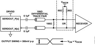
Figure 118. AC-Coupled Digital Output Termination Example
