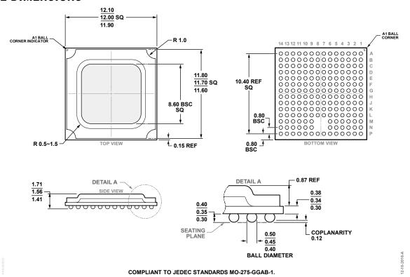
Figure 127. 192-Ball Ball Grid Array, Thermally Enhanced [BGA\_ED] (BP-192-1) Dimensions shown in millimeters
