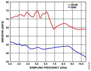
Figure 50. SNR/SFDR vs. Sampling Frequency,  $f_{\text{IN}} = 2600 \text{ MHz}$ , 10 GSPS
