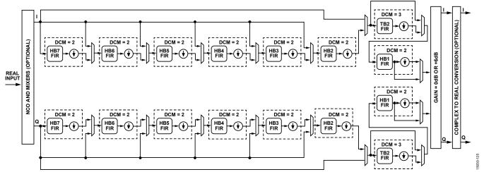
Figure 100. DDC Decimation Filter Block Diagram
