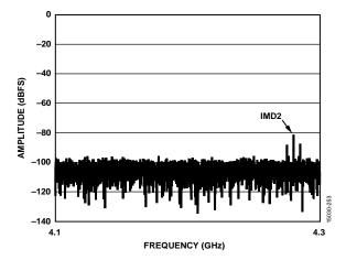
Figure 66. Two-Tone FFT, IMD2 Zoom In,  $f_{\rm IN1}=2137.5$  MHz,  $f_{\rm IN2}=2142.5$  MHz,  $A_{\rm IN1}$  and  $A_{\rm IN2}=-7$  dBFS (see Figure 65), 10 GSPS
