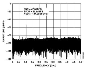
Figure 42. Single-Tone FFT with  $f_{\rm IN}$  = 5.5 GHz, 10 GSPS
