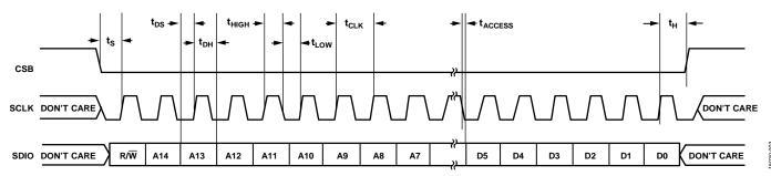
Figure 3. Serial Port Interface Timing Diagram (MSB First)
