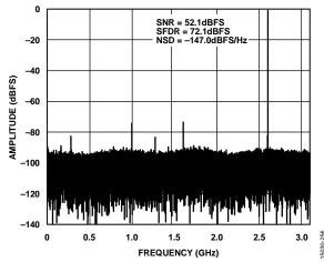
Figure 10. Single Tone FFT with  $f_{IN} = 2.6$  GHz, Sampling Frequency = 6.2 GSPS
