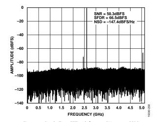
Figure 44. Single-Tone FFT with  $f_{IN} = 2.6$  GHz, 10.25 GSPS
