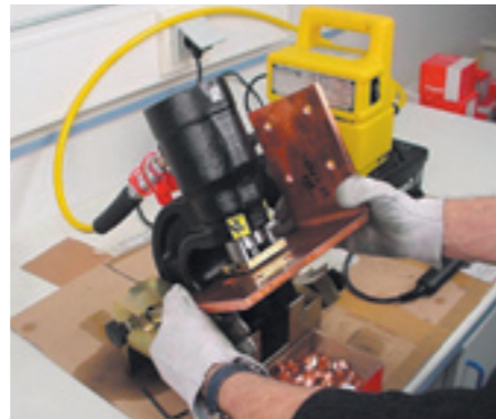
^ The hydraulic punch is used to make precision holes easily ... and with no chips
