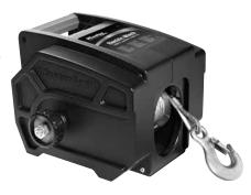
drum using a winch hook strap or hand saver bar. Always leave at least three turns of the cable on the winch drum to prevent the cable from pulling out of the winch.
