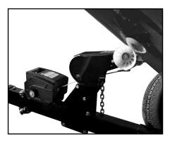
Your winch can generate 2,000lbs of pulling force so be sure that the mounting site selected can withstand a load well in excess of the 2,000lbs pulling force.
