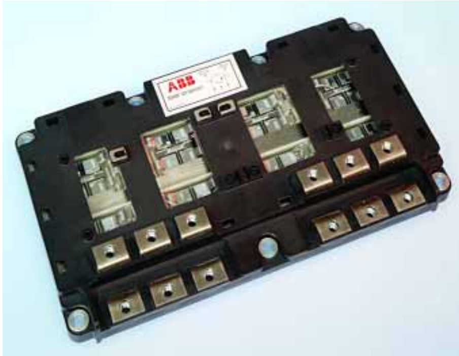
Fig.4: Photo of a 1200 Amp, 3300 V IGBT FLIP ® Module (Part No. 5SNB 12F3300D). The lids on top of the module have been removed to provide a view inside the module.
