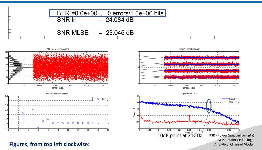
Recorded signal and PDF >> Post-processed signal at mid-stage point of the DSP >> PSD recorded signal single-side spectrum and estimated noise spectrum >> Channel Impulse Response (CIR)
