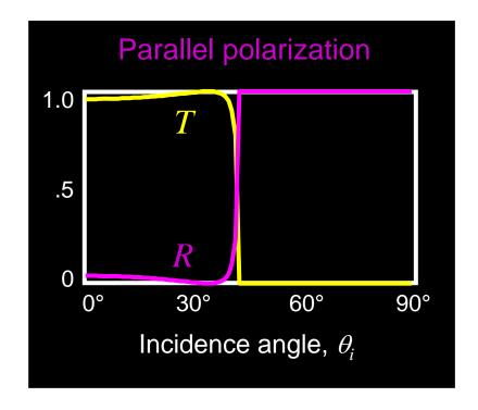
Note that the critical angle is the same for both polarizations.
