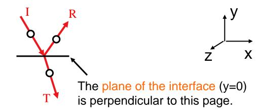
2. "P" polarization is the parallel polarization, and it lies **parallel** to the plane of incidence.
