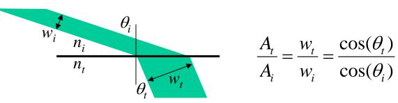
The beam expands (or contracts) in one dimension on refraction.
