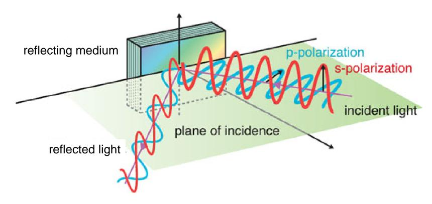
The amount of reflected (and transmitted) light is different for the two different incident polarizations.
