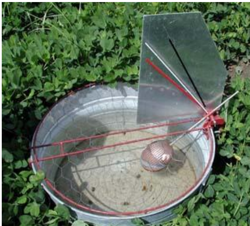
Figure 13.13. The University of GA EASY Pan that uses a pointer (white stick) to indicate when to irrigate (red line).
