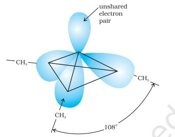
Fig. 13.1 Pyramidal shape of trimethylamine
