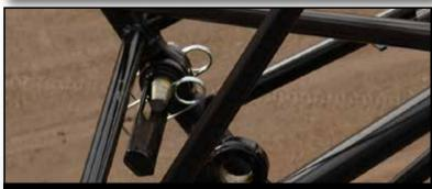
**Double tapered connecting pins** for installation/removal from outside of boom. Boom connecting pins store in pin catchers for transport.
