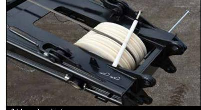
Quick reeve boom head Four polymer head sheaves with maintenance free sealed bearings
