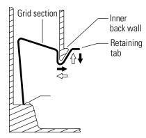
Figure 5-1. Protective Paper Catch Grid
