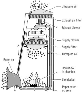
Figure 1-2. Airflow Filtering System
