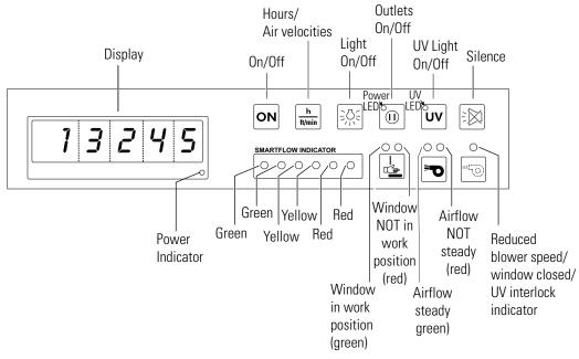
Figure 4-1. Control Panel Functions
