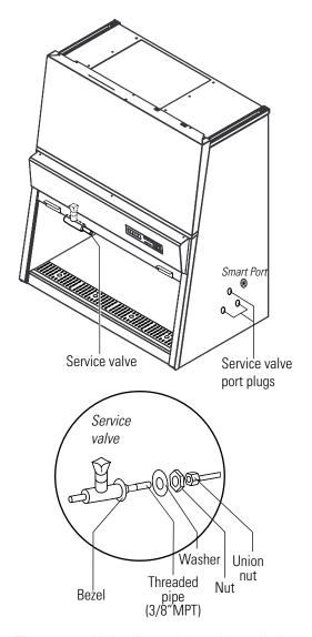
Figure 2-5. Valve Assembly and Installation
