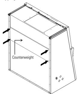
Figure 3-2. Unlocking the Counterweight
