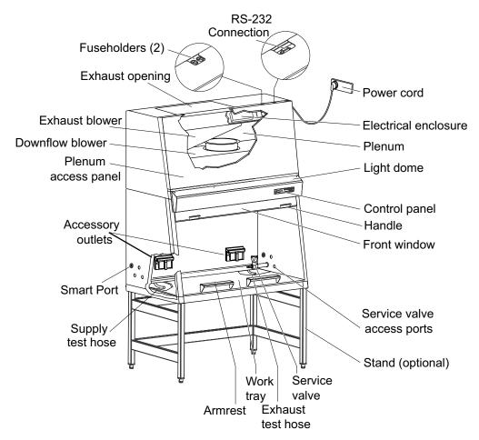
Figure 1-1. Unit Components
