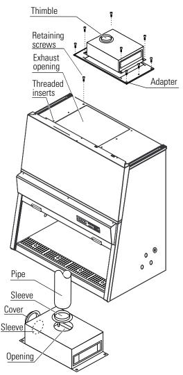
Figure 2-2. 6 ft Thimble and Sleeve
