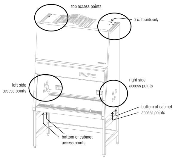
Figure 2-6. Possible Universal Piping Access Points
