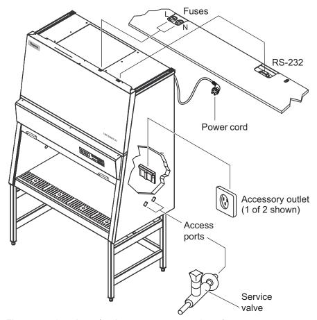
Figure 1-9. Interfaces (2 of 4 access ports are shown)
