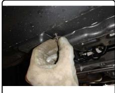
2. Raise hitch over exhaust and into position and loosely secure hitch with (4) M12 bolts and conical washers. Slide flat washers into position then 5/8" bolt through washer, bumper beam, and hitch securing with hex flange nut.
