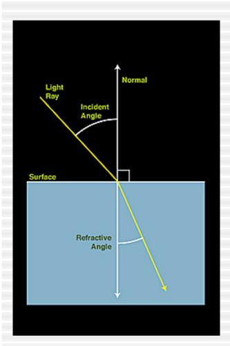
**Refraction** - to break or impair. The change in direction of a wave crossing a boundary between two different media. The different wave speed of the two media causes the bending. There is no returning wave.
