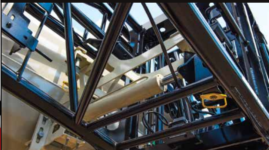
Fly erection and stowing assist cylinder
