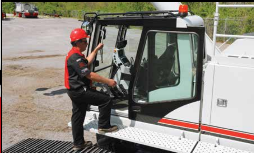
Non-slip safety strips, extended length catwalks, sideframe steps and upper guard rails provide sure-footed access to the crane upper.
