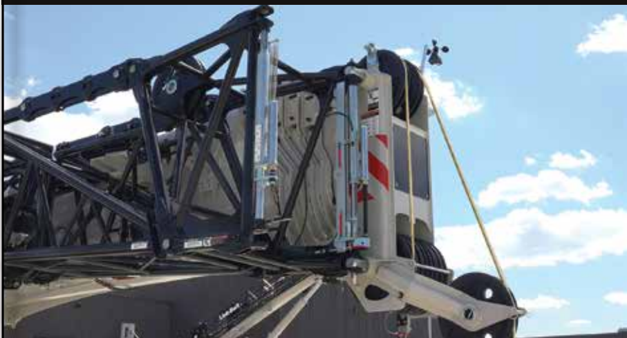
New efficient fly pinning design focuses on ease of assembly/disassembly
