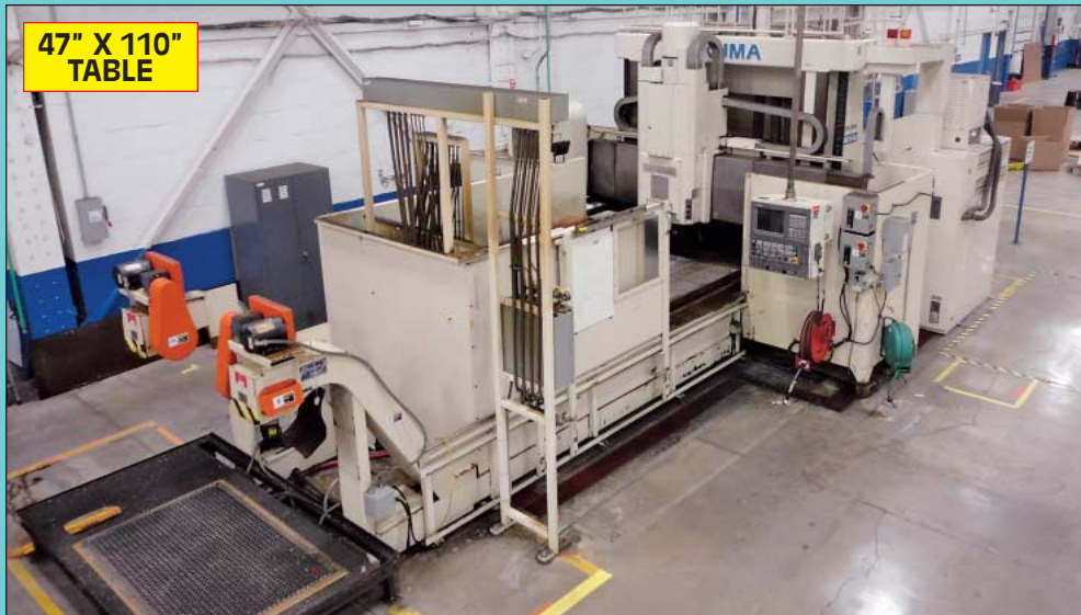
Okuma Model MCV-All 16X30 Double Column CNC Vertical Machining Center Bridge Mill (Installed 2002)
