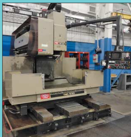
Enshu Model VMC-530 Heavy Die Mold Type CNC Vertical Machining Center
