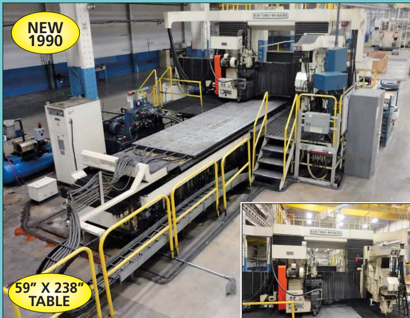
Sumitomo-Shibaura Type KEL-15 / KPL-1550-OG Double Column Bed Type CNC Surface and Way Grinder
