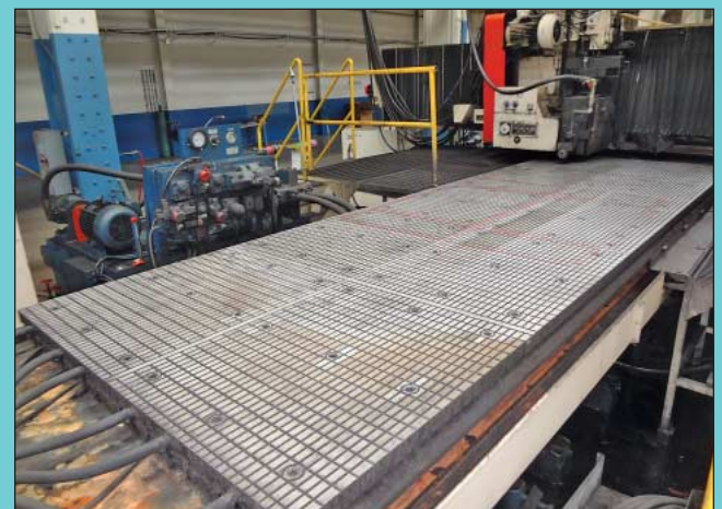
63" X 200" X 2" and 47" X 110" Thick Vac-U-Lok Vacuum Chuck Tables w/ 5 HP Vacuum Pump and Controls
