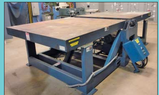
1,000 Lb. Per Side Cap. Foster 6' X 6' Two-Sided Hydraulic Tilting Weld Table
