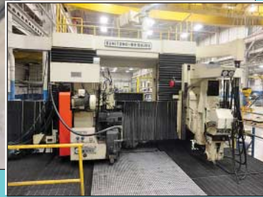
Sumitomo-Shibaura Type KEL-15 / KPL-1550-OG Double Column Bed Type CNC Surface and Way Grinder
