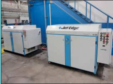
(2) 50 HP Jet Edge 55-50C Intensifier Pumps
