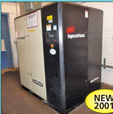
100 HP Ingersoll Rand Nirvana Model IRN100H-CC Rotary Screw Cabinet Enclosed Air Compressor
