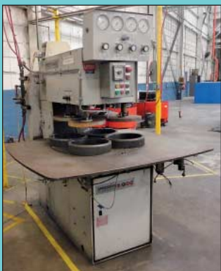
32" Dia. Speedfam Model G32BTGW 4-Station Lapping Machine
