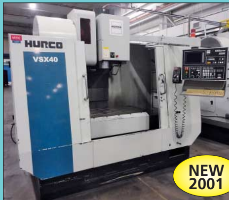
(2) Hurco Model VSX-40 CNC Vertical Machining Centers
