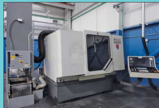
Walter Helitronic Type 45 CNC Cylindrical Grinder
