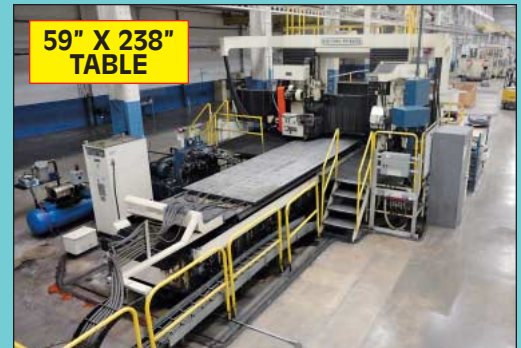
Sumitomo-Shibaura Type KEL-15 / KPL-1550-0G Double Column Bed Type CNC Surface and Way Grinder
