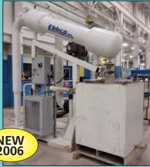
50 HP Ebbco Model GRS-0802-B Abrasive Removal System
