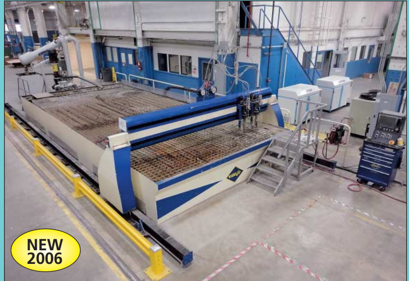
Ward-Jet Model R-3013 Two-Head CNC Water Jet Machine
