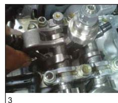
Once fastened the tool on the injector, tighten the pin with the impact mass to the dowel M10 and proceed with the injector extraction operating manually with impact mass (fig. 9).
