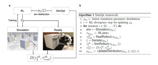
Figure 15.6: a. schematics for SimOPT. b. algorithm formulation of SimOpt.
