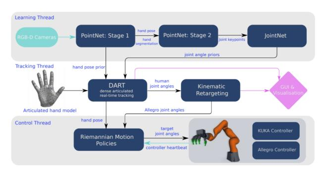
Figure 15.10: Method pipeline for DexPilot
