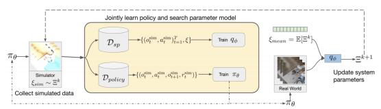
Fig. 2: Overall System: Using any off-the-shelf RL algorithm, we use simulated data to train both our policy and a Search Parameter Model (SPM)  $q_{\phi}$  which predicts whether a candidate set of system parameters  $\xi$  is higher or lower than those which produced an observed trajectory. We iteratively update our simulation by running our policy in the real world and using our SPM to predict which direction to update our simulator to make it closer to the real world.
