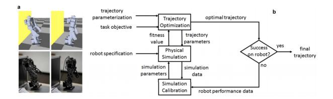
Figure 15.1: a. example of robot performing "Lean-to-Stand", top: training in simulation environment, bottom: testing in real world. b. Diagram for major component of the system.
