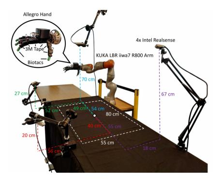
Figure 15.9: System setup for teleoperation. The human performs actions in a human arena (on the bottom right), and the robot replicates these actions (on the top left). The four RGB cameras obtain a multi-view coverage of the space at the appropriate distance. The tactile sensors on the Allegro hand are not used in this project, but in the future they could facilitate data collection for imitation learning.
