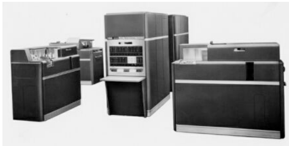
This "white room" view of a 650 installation shows an IBM 533 Card Read Punch in the foreground at left; the 650 Console Unit at center, with an IBM 655 Power Unit behind it; and an IBM 537 Card Read Punch at right. (IBM Archives)
