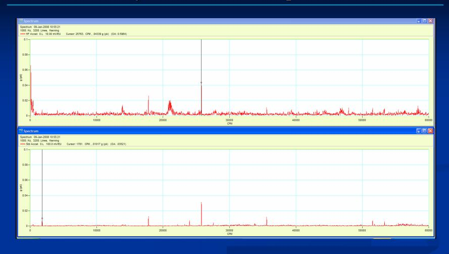
Note the difference in the noise floor of a 10 mV/g vs. 100 mV/g
