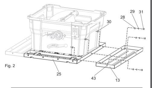
**NOTE:** Only one hole [42,43] on the side of the extension tables must be in the front after finished.
