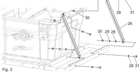
> Attach two supporting bars [26] and hose hold [18] with the right extension table with flat washers 6 [28], spring washers 6 [29], hex nuts M6 [30] and hex bolts M6 x 16 [31].
