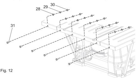
> Push on the front guide rail [11] with slot of the front guide rail aligned with the six hex nuts M6 [30] as shown in the Fig. 13.
