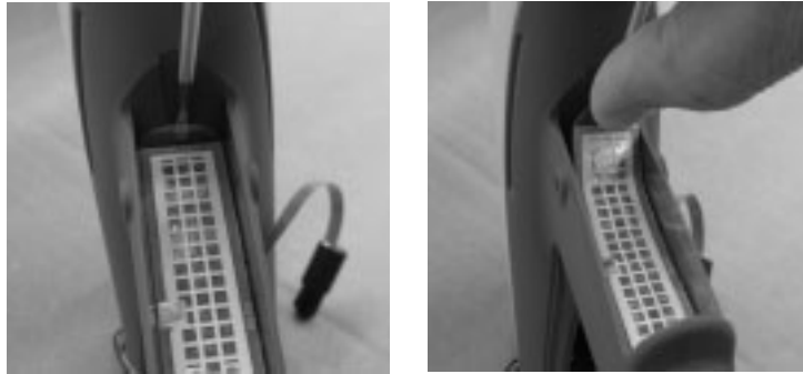
Figure 6-8 Removing the Trigger Switch from the Handle
