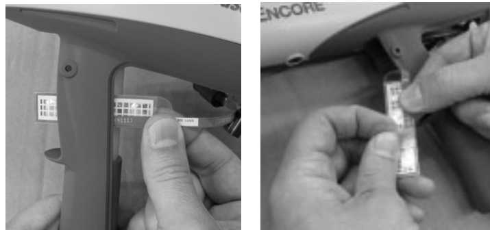
Figure 6-9 Installing the Trigger Switch – Steps 1 and 2
