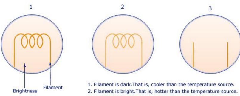
Filament disappears. Thus, equal brightness between filament and temperature source.
