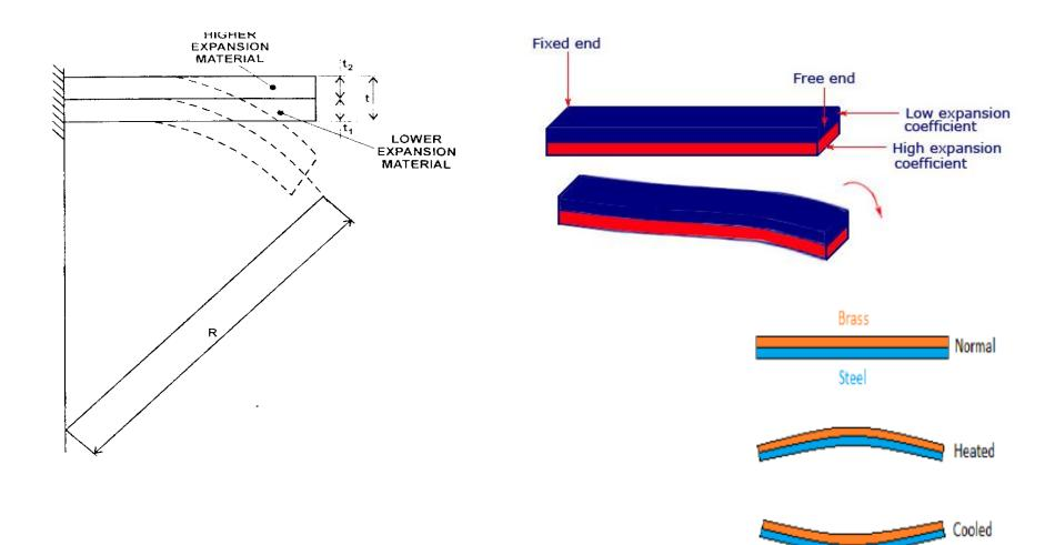
Important properties of material for selection of bimetallic thermometers. (these properties should be high)
