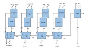
Fig.7 The Proposed16-Bit Half Adder Based SQRT CSLA Using CBL
