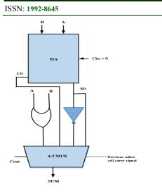
FIG.6 Half Adder With Common Boolean Logic
