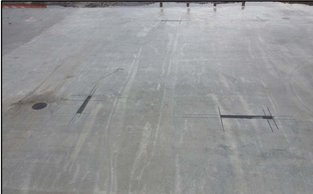
Figure 26. Slots in Test Section to Evaluate Segregation
