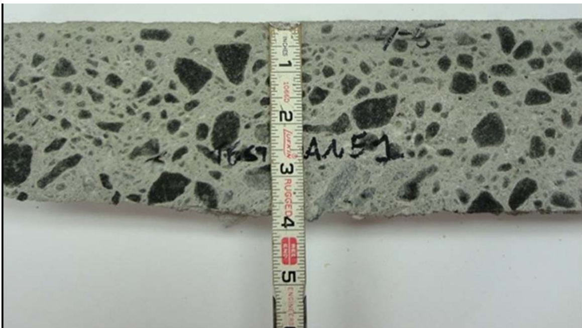
Figure 28. Example of Segregation and Excess Surface Paste with Traprock
