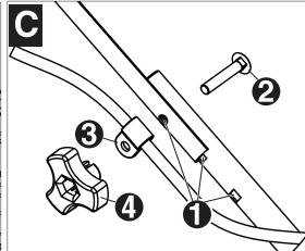
and grass bag. Insert carriage bolt and install knob for other side.
