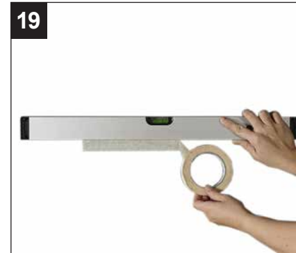
Measure and mark 160 cm. Make sure it is level.
