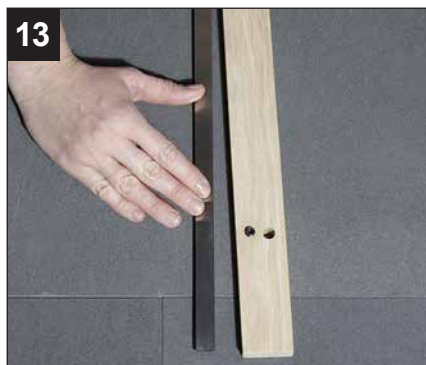
TIP: the slide with holes in it goes on top. Remove the metal bar inside the wooden slides.
