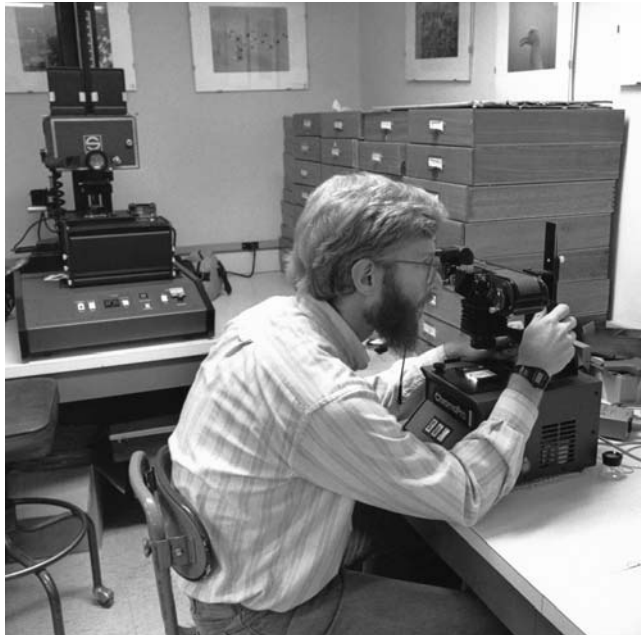
VIREO is equipped with small- and large-volume slide duplicators. In-house duplication allows consistent quality-control, reduces costs, and, most importantly, avoids the possibility that originals will be damaged or lost if sent out for duplication.
