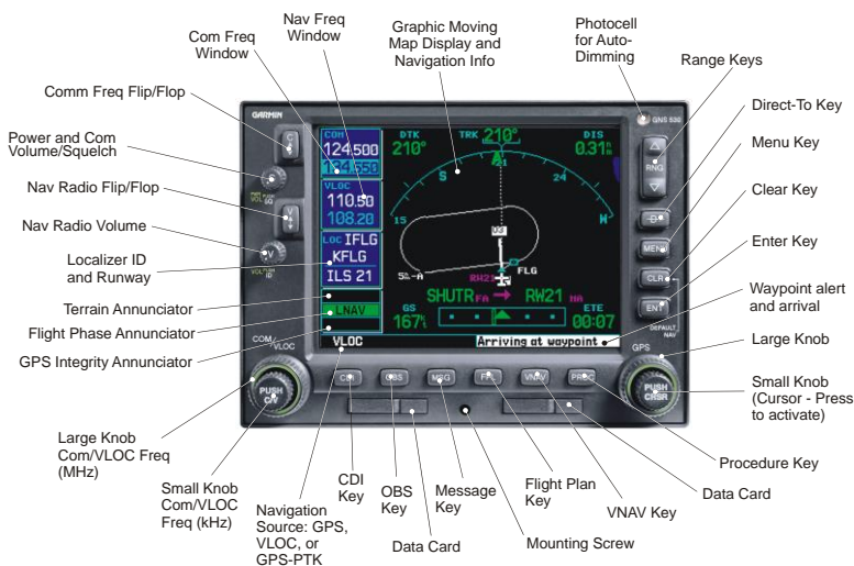
Figure 1 - 500W Series Control and Display Layout
