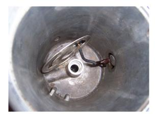
Set the heater element sideways into the fuel bowl. This will allow you to reach in and plug the element into the electrical connector with your hand or by using a pair of needle nose pliers.
