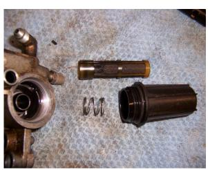
The 1994-1995 models have a screen filter canister that is attached to the FPR. It simply unscrews from the FPR. The screen element slips over the tube that is cast into the FPR and the spring that sits in the bottom of the canister holds it in place. You will want to use a soft bristle brush to thoroughly clean the filter and blow drv with compressed air.
