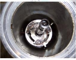
**Remove the Fuel Bowl Heater Element:** To remove the element you will need a 7/8" crowsfoot wrench. The black filter stand pipe must be removed by un-screwing it from the fuel bowl. It is a **left hand thread** and once you break it loose it will unscrew by hand. Once you remove the stand pipe, you can reach into the bowl with a pair of needle nose pliers and disconnect the heater's electrical plug.
