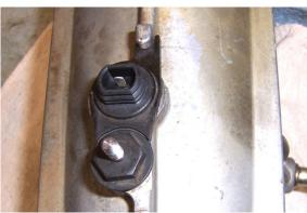
After cleaning the Water In Fuel Sensor, use the **O-ring #6**. Lube the o-ring area with some light oil or motor oil and screw it back into the WIF port below the Heater connector.
