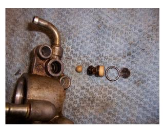
Be very careful removing the bleeder orifice as there is a check ball sitting in the recess below it. This check ball has a lot of bounce and will be difficult to locate if it falls out and decides to leave. In this photo you can see the check ball, bleeder orifice with the two o-rings, the sealing o-ring between the FPR and the fuel bowl body and the screen.
