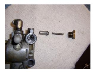
The main FPR seat valve is straight forward seat, spring and cap in that order. Install the new o-ring on the brass FPR cap (use the **O-ring #8)**. Lube the o-ring area with some light oil or motor oil and screw it into the port making sure the spring is center on the pointed spike on the brass plug.
