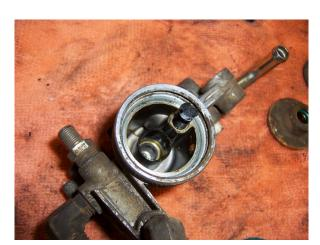
(96-97 Only) There is a plastic snubber that is in the port leading to the Fuel Restriction Sensor that can be removed by gently prying it out with a pick tool. This will open the internal port for additional cleaning.
