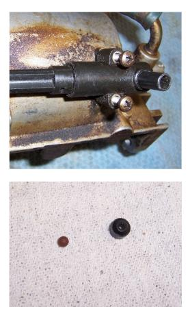
**Remove the Fuel Drain Valve:** Use a #2 Phillips screwdriver and remove the 2 machine screws that hold the valve to the bowl. The extension handle will separate from the valve once the unit is removed. The keyway is configured so the handle extension will only couple with the valve in one position so there is no need to be concerned with handle orientation. Set the drain valve aside to be cleaned with the other parts.
