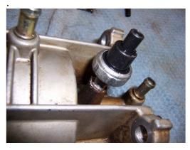
**Remove the Fuel Restriction Sensor:** This sensor is threaded into the Fuel Bowl pressure line. On the 94-95 models it is at the bottom of the bowl while the 96-97 models have it threaded into the Fuel Pressure Relief body. Set the sensor to the side to be wiped clean as it should not be submerged in cleaning solvent. **When reinstalling this sensor, do not over**
