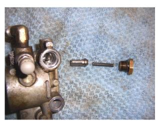
Here is the Fuel Pressure Relief Valve removed from its containing port. There are only three parts to this valve, the seat, spring and brass cap. Set all these parts aside to be cleaned in the parts cleaner tray.
