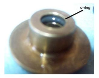
(96-97 models Only) Here is the **O-ring #3** inserted into the recess in the FPR base plate that seals the hard line to the FPR.
