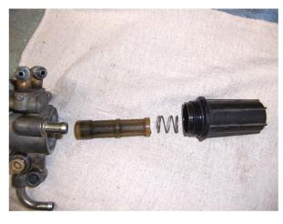
This is the Filter screen canister for the **94-95** models. The canister will use the **O-ring #9**.
