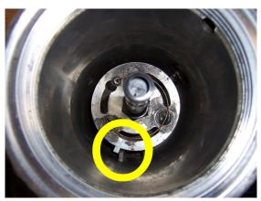
Place the heater element on the stand pipe port with the tab of the element plate **to the left** of the aluminum tab cast into the fuel bowl. These tabs keep the heater element from turning while tightening the stand pipe and causing damage to the electrical wire and connector.
