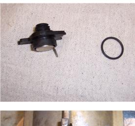
After cleaning the Heater electrical connector, use the **O-ring #4**. Lube the o-ring area with some light oil or motor oil and insert it back into the heater port on the fuel bowl. Rotate the connector so the tall tab interlocks under the tab cast in the fuel bowl.
