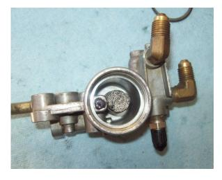
(96-97 Only) When removing the c-clip and plate from the regulator assembly, the filter is exposed. This filter can be removed and washed in solvent until the fluid runs clean.
