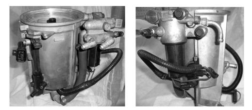
You can now remount the fuel bowl in the engine bay and reconnect the wiring harness and fuel hoses. It will be necessary to connect the hose attached to the bottom of the fuel bowl prior the bolting the bowl to the engine.
