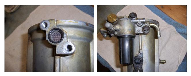
Place the cleaned screen filter into the port opening on the fuel bowl and set the new **O-ring #5**.into the recess.
