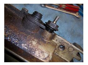
**Remove the Fuel heater electrical connector & Water in fuel Sensor**: The Water in Fuel sensor will unscrew from the fuel bowl by using a 9/16" box end wrench. Set it aside to be cleaned with other parts later.
