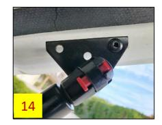
20. Using the bracket as a guide, drill the second hole, and install the second rivet to complete the bracket installation (**Fig 15**).
