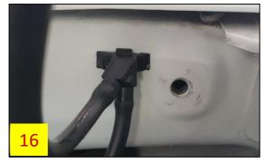
c. Tie the windshield washer hose to a secure location away from or behind the passenger side ball stud with a zip tie or other means (ABS module is a convenient tie down location, see Fig 17). If you have the buzzer bracket on the passenger side, you can drill a hole in that bracket and snap the washer tube connector into it, as shown in Fig 8. In high lift configurations, you may need to extend or replace the existing washer vacuum tube with a longer section of 3/16" vacuum tubing.
