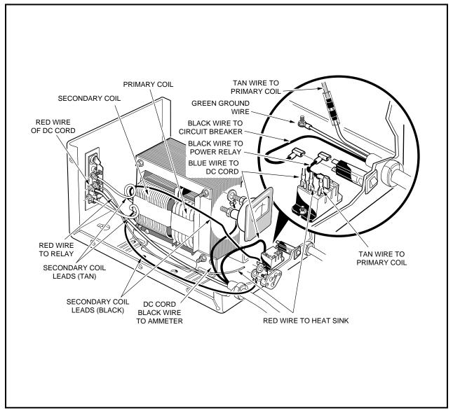
Figure 14-6 PowerDrive Battery Charger
