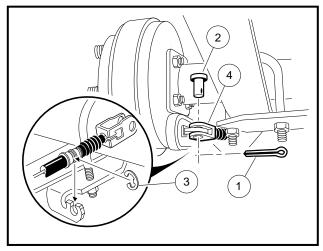
Figure 16-9 Disconnect Brakes
