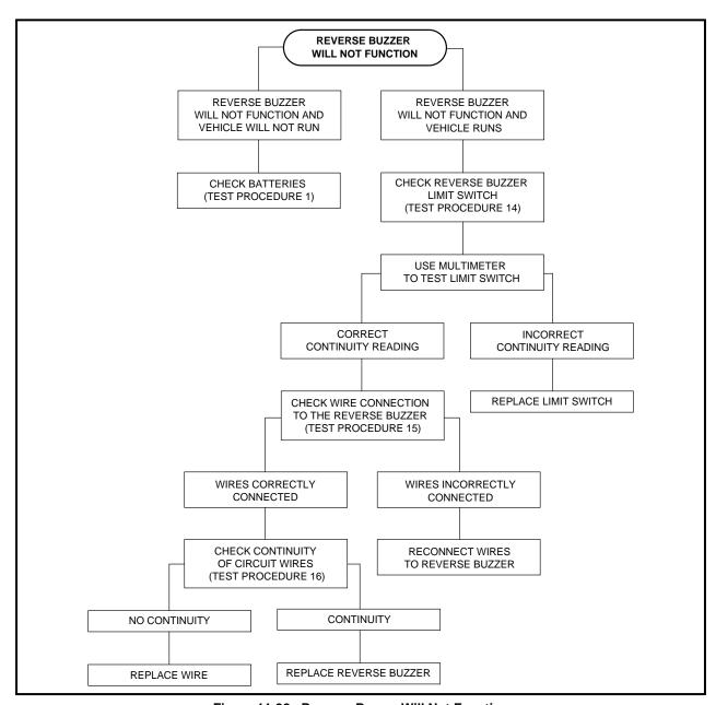
Figure 11-32 Reverse Buzzer Will Not Function
