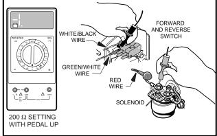
Figure 11-13 Test Limit Switch (Multi-step)
