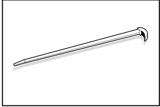
Figure 16-2 Rolling Wedge Bar
