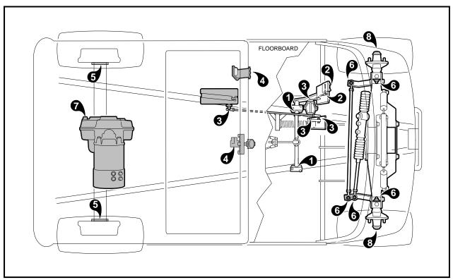
Figure 10-2 Vehicle Lubrication Points-DS, Tourall, Fairway Villager and Carryall I
