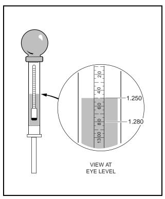
Figure 13-8 Hydrometer
