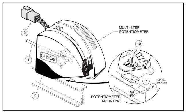
Figure 12-14 Multi-step Potentiometer Mounting
