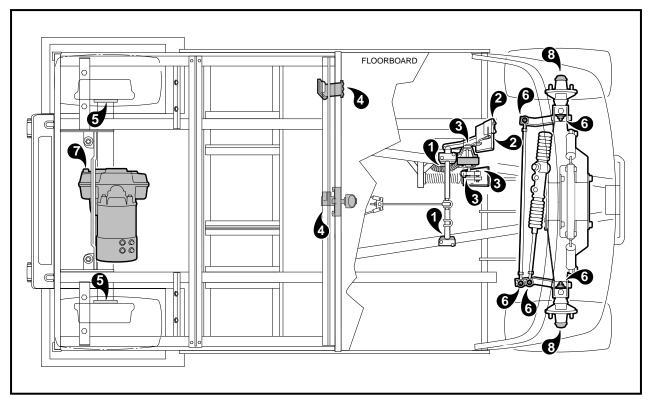
Figure 10-3 Vehicle Lubrication Points-Carryall II, Carryall VI, Trans-porter, Trans-sender, Resort Villager
