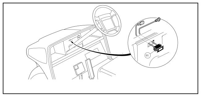
Figure 12-16 Battery Warning Light
