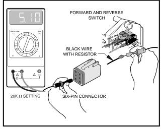
Figure 11-30 Test Half-Speed Reverse Limit Switch
