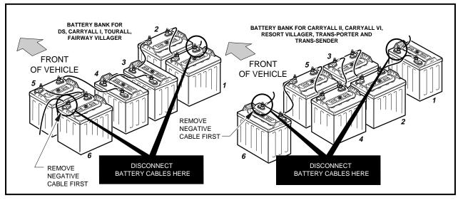
Figure 12-1 Battery Configuration
