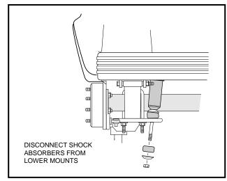
Figure 16-10 Disconnect Shocks
