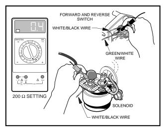
Figure 11-12 F&R Anti-Arcing Limit Switch
