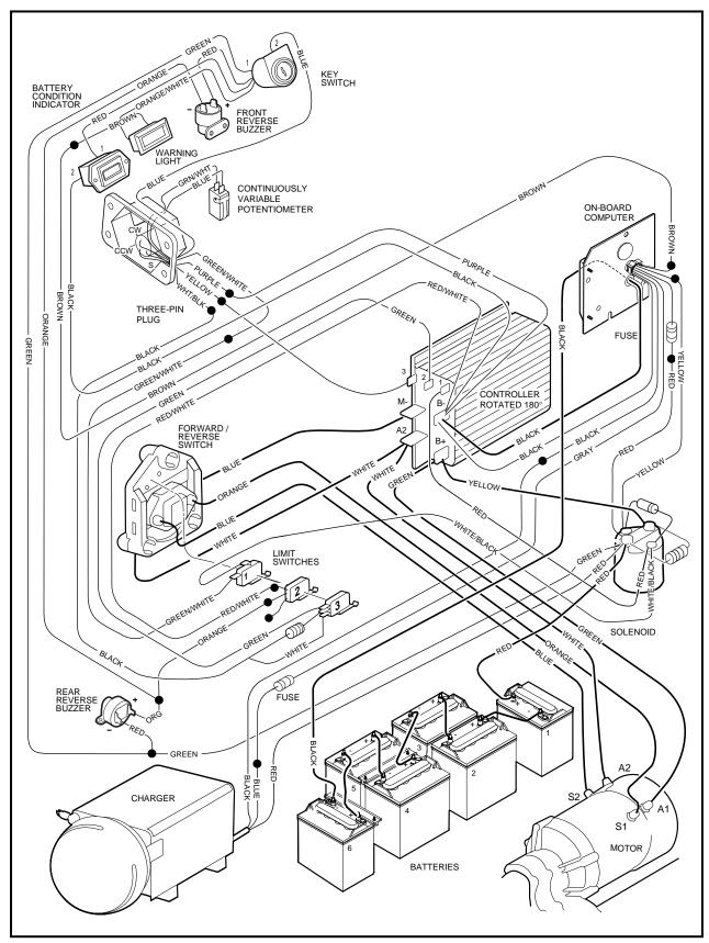
Figure 11-5 Wiring Diagram - Carryall VI, Trans-Porter/Trans-Sender
