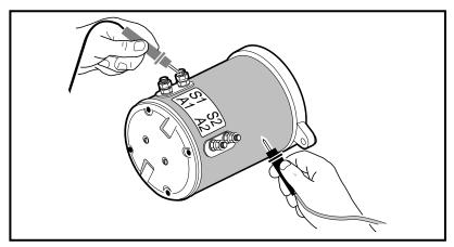
Figure 15-2 Test for Motor Short Circuits
