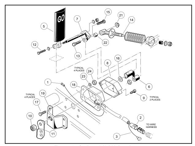
Figure 12-11 Continuously Variable Potentiometer
