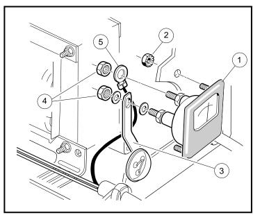
Figure 14-21 Ammeter Replacement
