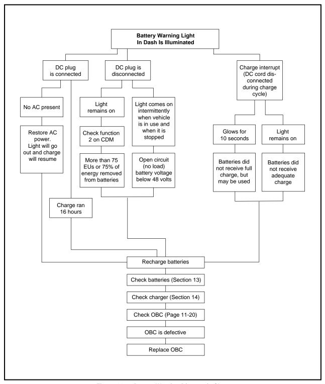
Figure 11-7 Battery Warning Diagnostic Chart
