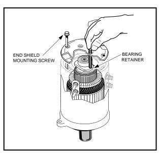
Figure 15-16 End Shield Installation
