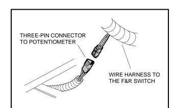
Figure 11-25 Three-Pin Connector
