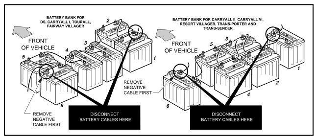
Figure 11-1 Battery Configuration
