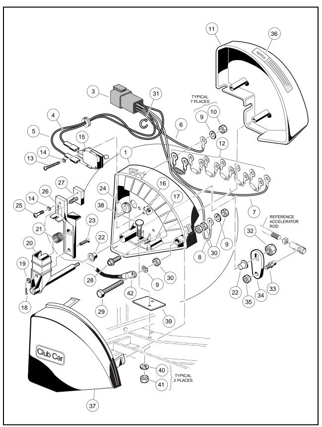
Figure 12-13 Multi-step Potentiometer
