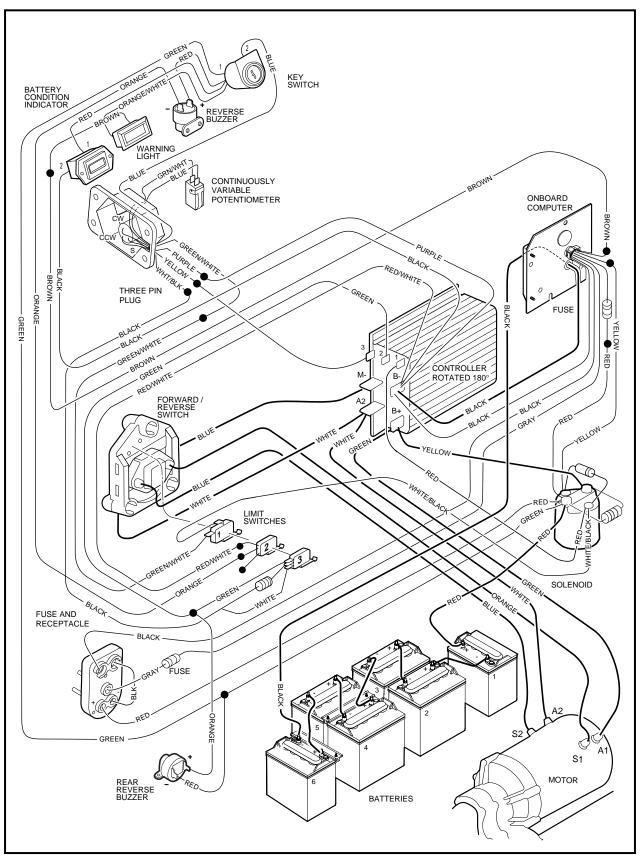
Figure 11-6 Wiring Diagram - Resort Villager
