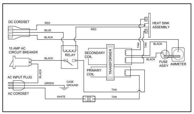
Figure 14-5 PowerDrive Battery Charger Wiring Diagram
