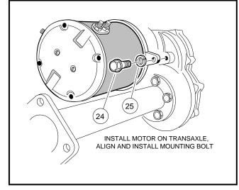
Figure 15-17 Motor Installation
