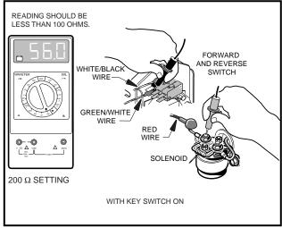
Figure 11-11 Test Key Switch (All Electric Vehicles)
