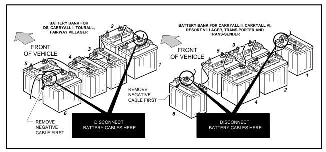
Figure 13-5 PowerDrive Battery Configuration
