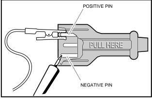
Figure 14-15 DC Plug Test Leads
