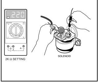
Figure 11-15 Test Diode
