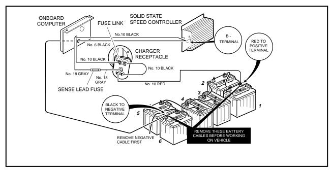
Figure 14-2 Charge Circuit and Battery Configuration - Short Frame Vehicle
