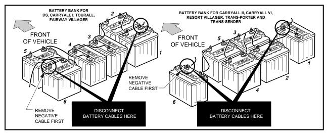
Figure 10-1 Batteries
