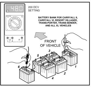
Figure 11-9 Battery Test - Long Frame Vehicle
