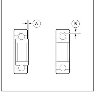
Figure 15-12 Check Brush Spring Tension
