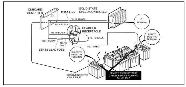
Figure 14-3 Charge Circuit and Battery Configuration - Carryall II and Long Frame Vehicles With Charger Receptacles.
