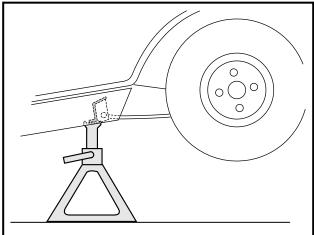
Figure 16-8 Support Vehicle on Jackstands
