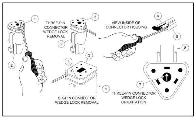
Figure 12-4 Terminal Plug Housing
