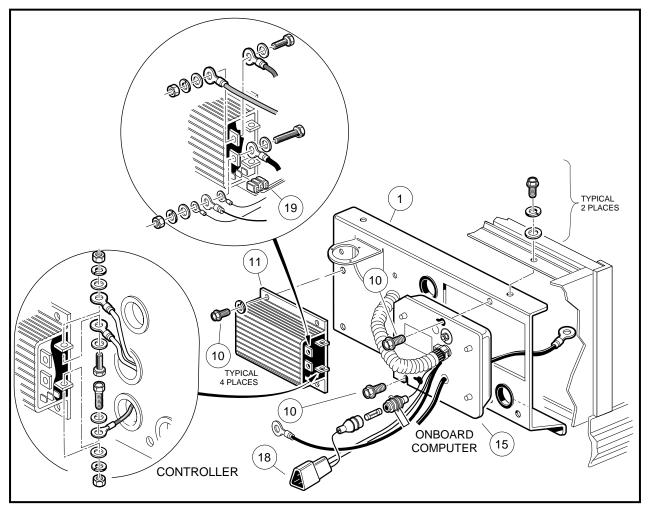
Figure 12-8 Controller and Onboard Computer - Long Body Vehicles
