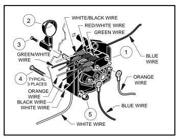
Figure 12-2 F&R Switch Wiring
