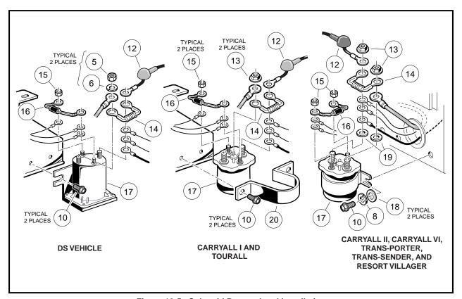
Figure 12-5 Solenoid Removal and Installation
