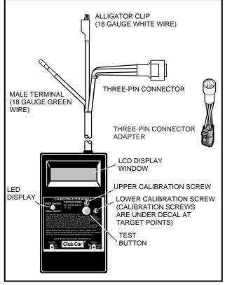
Figure 11-23 Test Multi-step Potentiometer
