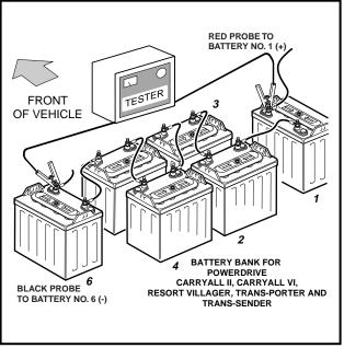
Figure 13-9 Discharge Test - Battery Configuration A Figure 13-10 Discharge Test - Battery Configuration B
