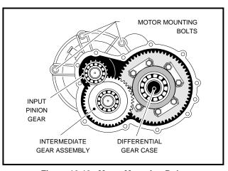
Figure 16-13 Motor Mounting Bolts
