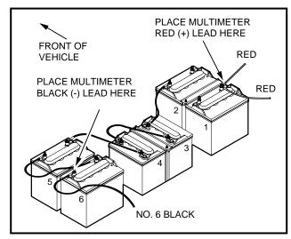
Figure 14-9 Battery Pack - Short Frame Vehicle
