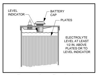
Figure 13-6 Battery Electrolyte Level
