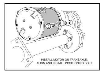
Figure 16-14 Motor Positioning Bolt
