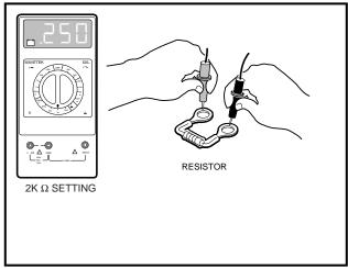
Figure 11-21 Test Solenoid Contacts
