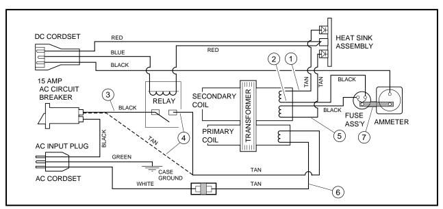
**Figure 13-11 PowerDrive Charger Wiring Diagram**
