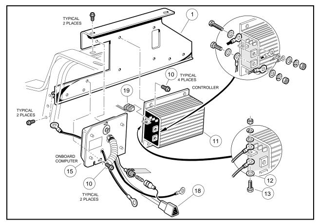
Figure 12-7 Controller and Onboard Computer - DS, Tourall and Carryall I Vehicles
