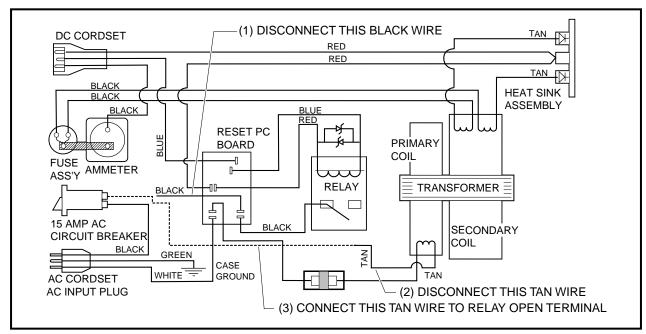
Figure 13-12 Onboard PowerDrive Charger Wiring Diagram
