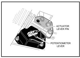
Figure 12-10 Potentiometer Housing
