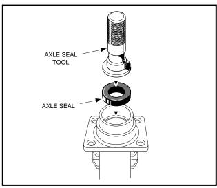
Figure 16-7 Axle Seal Tool
