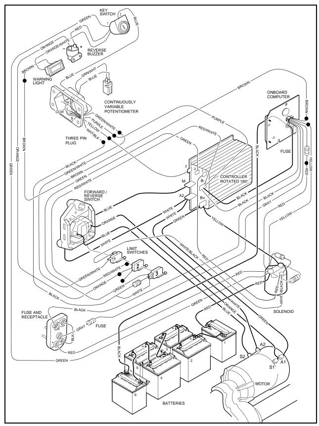
Figure 11-4 Wiring Diagram - Carryall II
