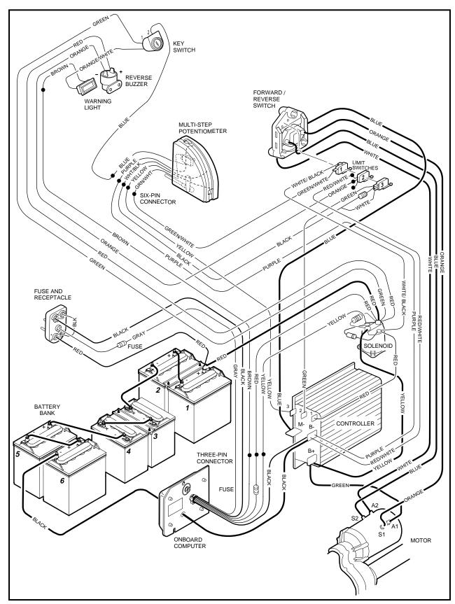
Figure 11-2 Wiring Diagram - DS Electric Vehicle
