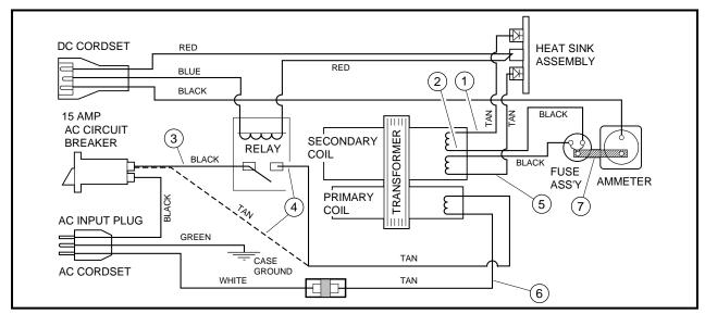
Figure 14-17 Test Transformer Wiring Diagram
