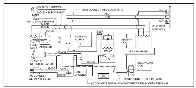
Figure 14-28 Onboard Charger Wiring Diagram
