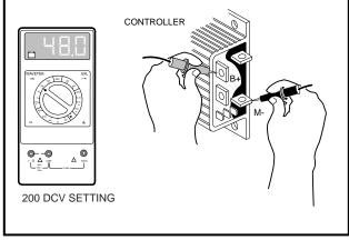
Figure 11-26 Test Input Voltage
