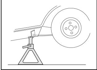
Figure 15-3 Lift Vehicle with Floor Jack
