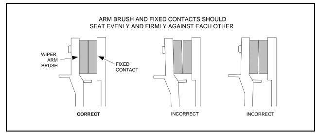
Figure 12-12 Multi-step Potentiometer Arm Brush and Fixed Contacts
