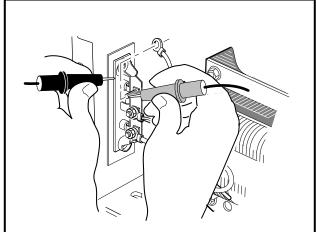
Figure 14-14 Diode Test, Reverse Probe Position
