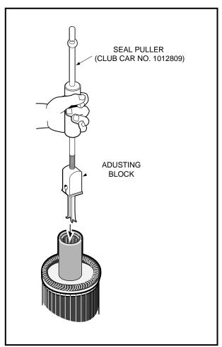
Figure 15-10 Guide Ring Removal
