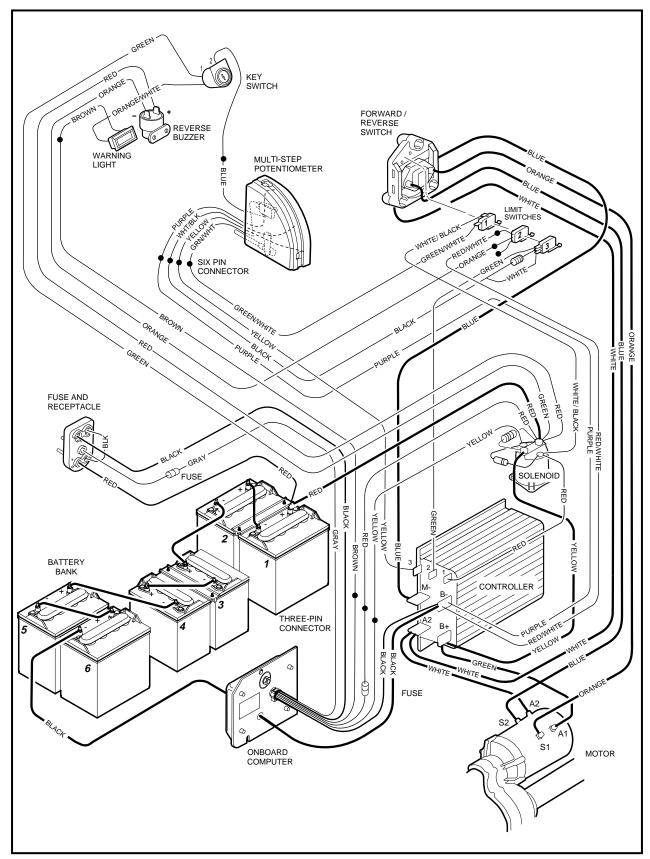
Figure 11-3 Wiring Diagram - Tourall, Carryall I
