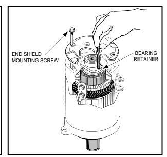
Figure 15-16 End Shield Installation
