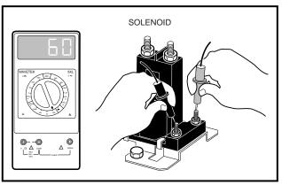
Figure 11-8 Solenoid Activating Coil Test
