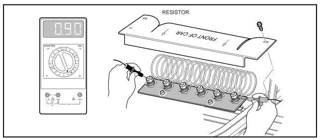
Figure 11-11 Resistor Test
