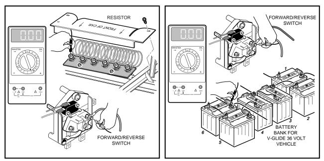
Figure 11-17 Motor Test - Armature
