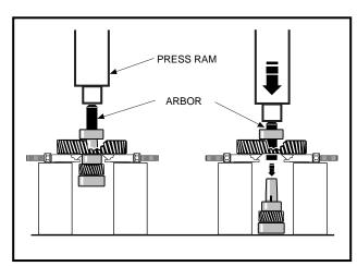
Figure 16-15 Intermediate Gear Assembly
