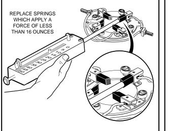
Figure 15-6 Brush Spring Tension
