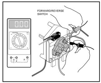
Figure 11-12 F&R Switch Test - Step 1.1
