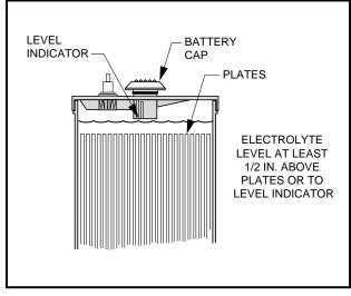
Figure 13-6 Battery Electrolyte Level
