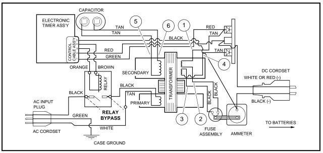
Figure 14-13 Relay Bypass Wire Placement
