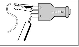
Figure 14-12 Charger DC Plug, Reverse Probes
