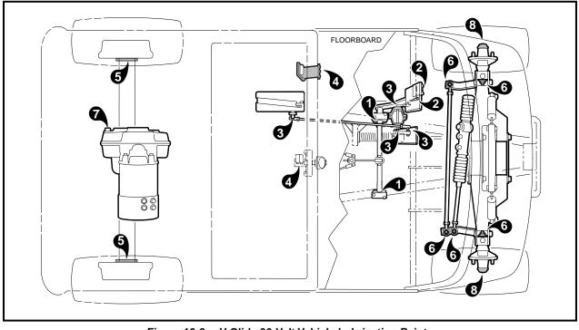
Figure 10-2 V-Glide 36-Volt Vehicle Lubrication Points
