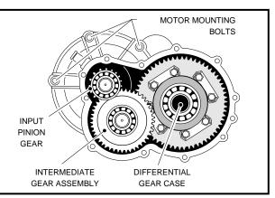
Figure 16-13 Motor Mounting Bolts
