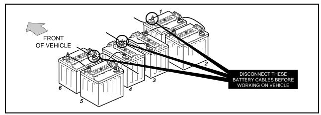
Figure 12-1 V-Glide Battery Configuration
