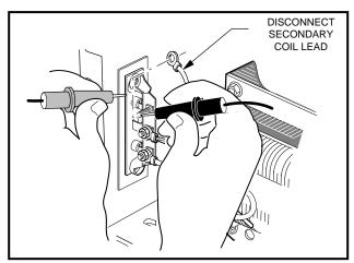
Figure 14-9 Single Diode Test
