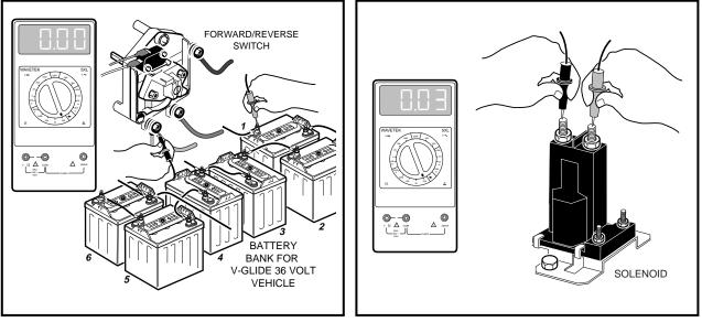
Figure 11-20 Solenoid Contacts - Power On, Step 1 Figure 11-21 Solenoid Contacts - Power On, Step 2
