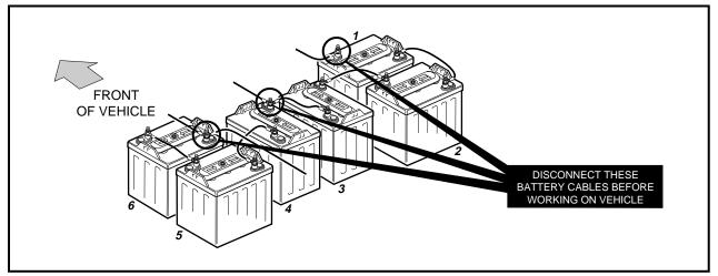
Figure 10-1 V-Glide Battery Configuration
