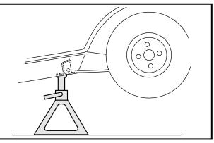
Figure 15-4 Support Vehicle on Jackstands
