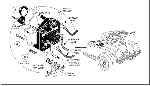
Figure 12-10 Removal and Installation of the F&R Switch
