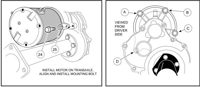
Figure 15-17 Motor Installation
