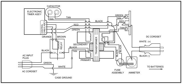
Figure 14-2 Charger Wiring Diagram
