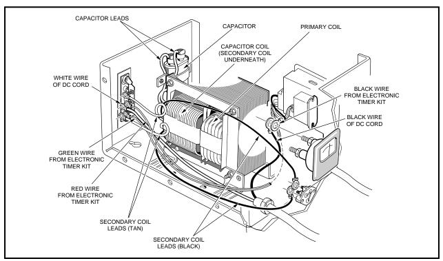
Figure 14-3 Charger Wiring
