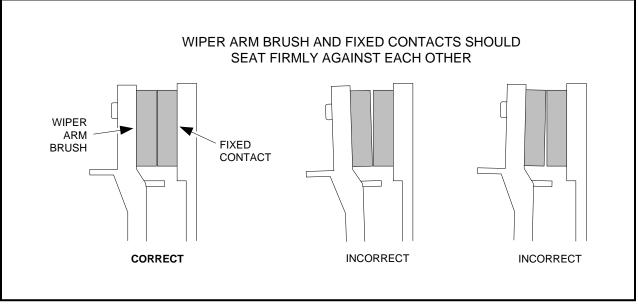
Figure 12-7 Wiper Switch Arm Brush and Fixed Contacts
