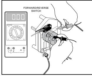
Figure 11-14 F&R Switch Test - Step 1.3
