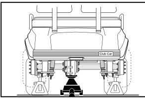
Figure 15-3 Support Transaxle on Floor Jack
