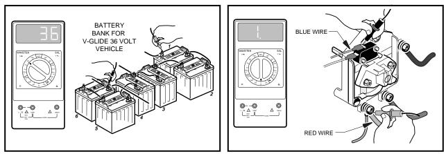
Figure 11-4 Batteries/Voltage Test
