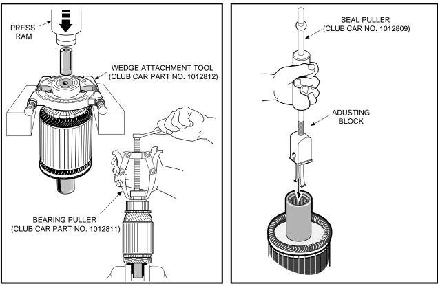
Figure 15-10 Bearing Removal
