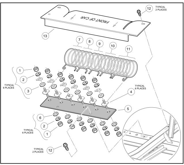
Figure 12-6 Mounting Board and Resistors
