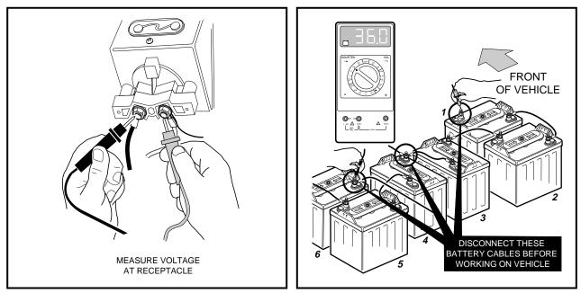
Figure 14-6 Voltage at Receptacle
