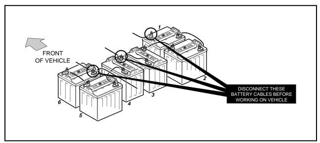
Figure 15-1 V-Glide 36-Volt Battery Configuration
