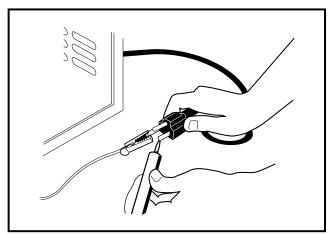
Figure 14-8 Test AC Plug Blades
