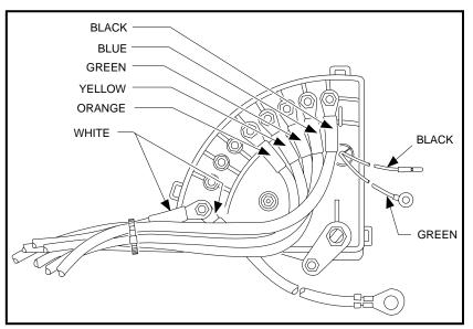
Figure 12-9 V-Glide Wiper Switch Wires
