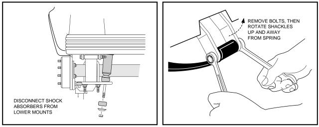
Figure 16-10 Disconnect Shocks
