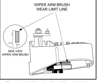
Figure 11-22 Wiper Arm Brush and Fixed Contacts
