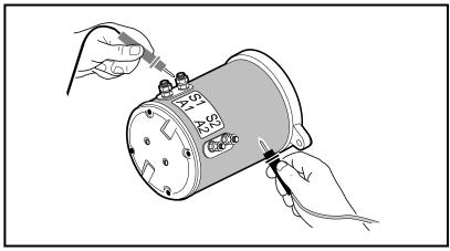
Figure 15-2 Test for Motor Short Circuits
