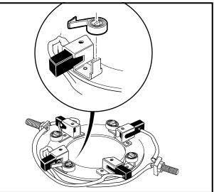
Figure 15-7 Brush Spring Removal
