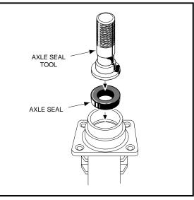
Figure 16-7 Axle Seal Tool
