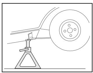
Figure 16-8 Support Vehicle on Jackstands
