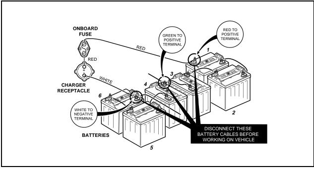
Figure 14-4 Charge Circuit
