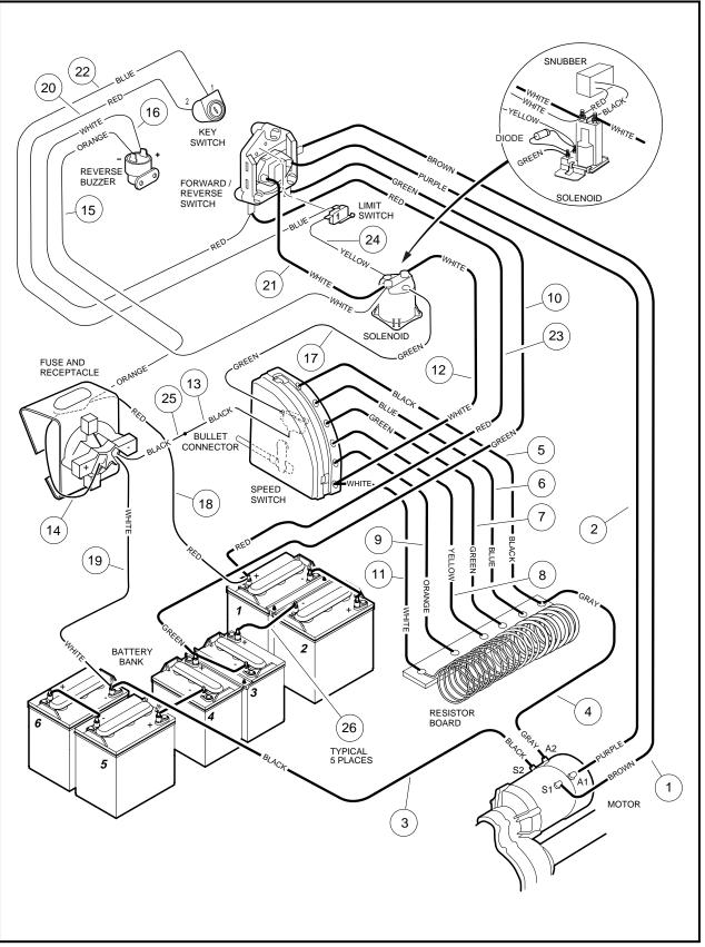
Figure 11-3 Vehicle Wiring Diagram
