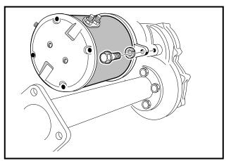
Figure 16-14 Motor Positioning Bolt
