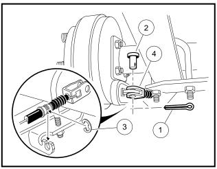
Figure 16-9 Disconnect Brakes
