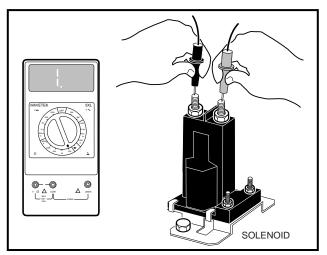
Figure 11-19 Solenoid Contacts - Power Off
