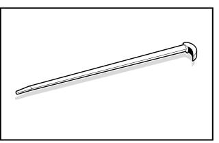
Figure 16-2 Rolling Wedge Bar
