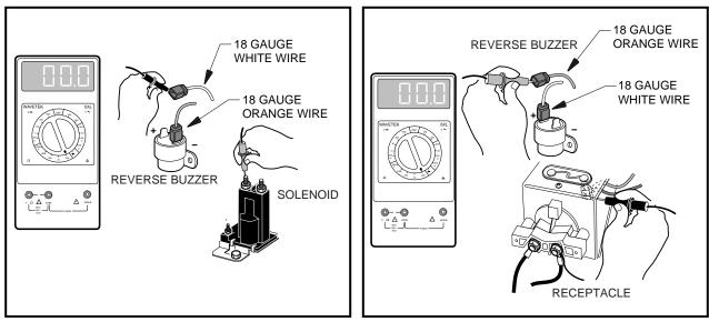
Figure 11-9 Reverse Buzzer Test - White Wire
