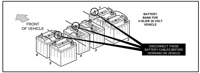
Figure 11-1 V-Glide Battery Configuration
