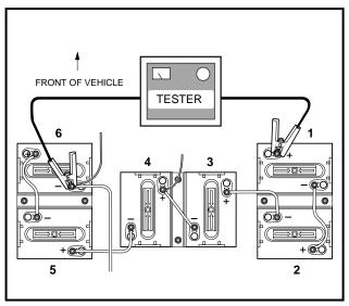
Figure 13-9 Discharge Test
