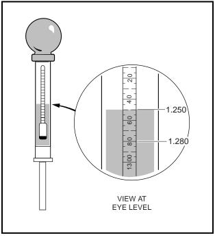
Figure 13-8 Hydrometer
