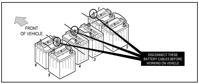
Figure 13-5 V-Glide 36-volt Battery Configuration
