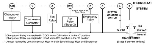
Figure 2. Typical wiring diagram for single transformer systems
