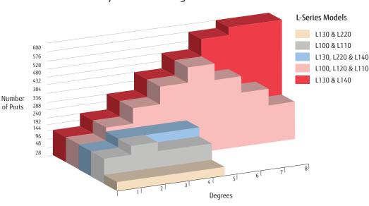
L-series blades can be deployed in multiple combinations to get the desired add/drop port counts per degree. This table assumes a 50 GHz channel.
