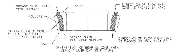
Figure 313 - Packing Bearing Cones
